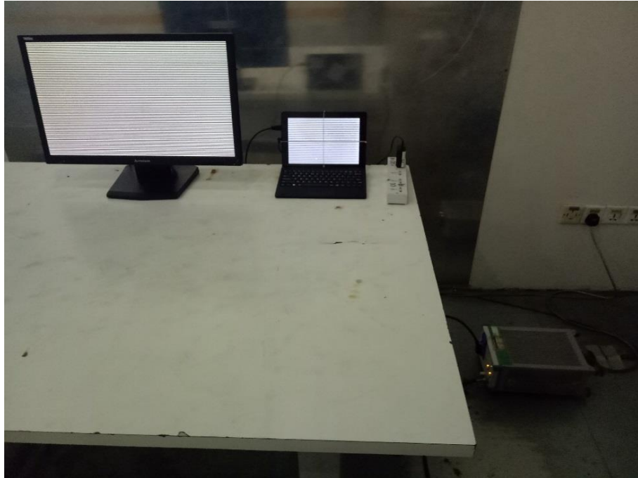
Photograph 1: Set-up for Conducted Emission
