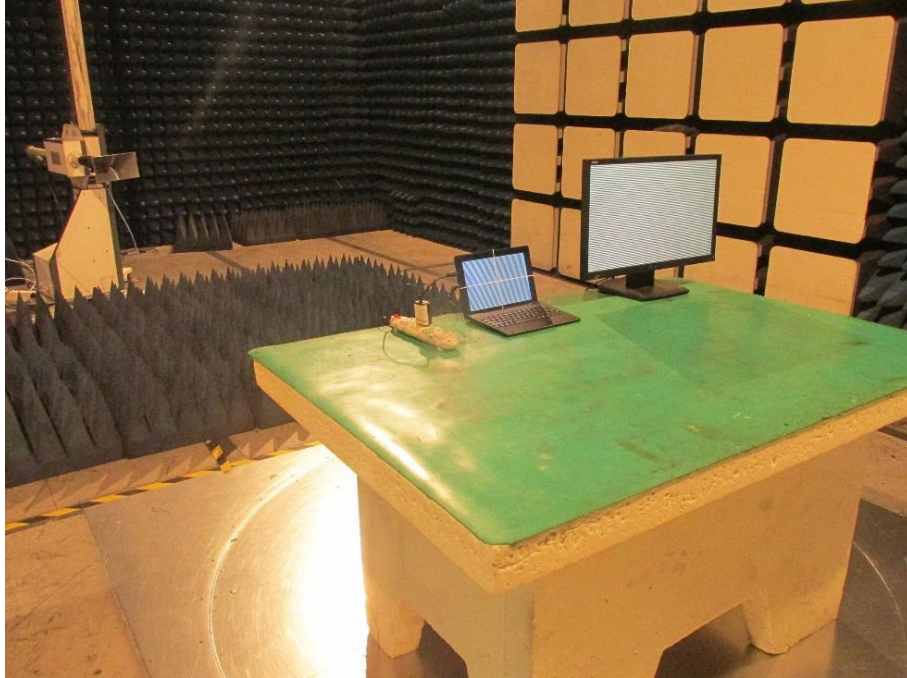
Photograph 3: Set-up for Radiated Emission (above 1GHz)
