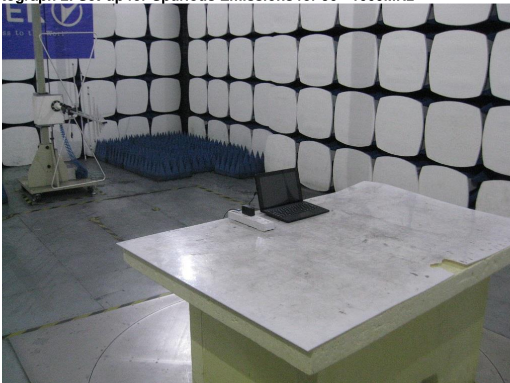
Photograph 2: Set-up for Spurious Emissions for 30 - 1000MHz
