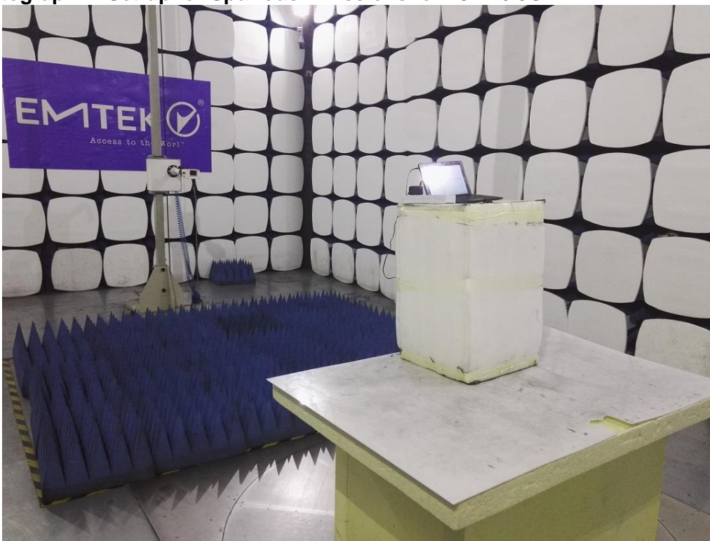
Photograph 4: Set-up for Spurious Emissions for 18 - 26.5GHz
