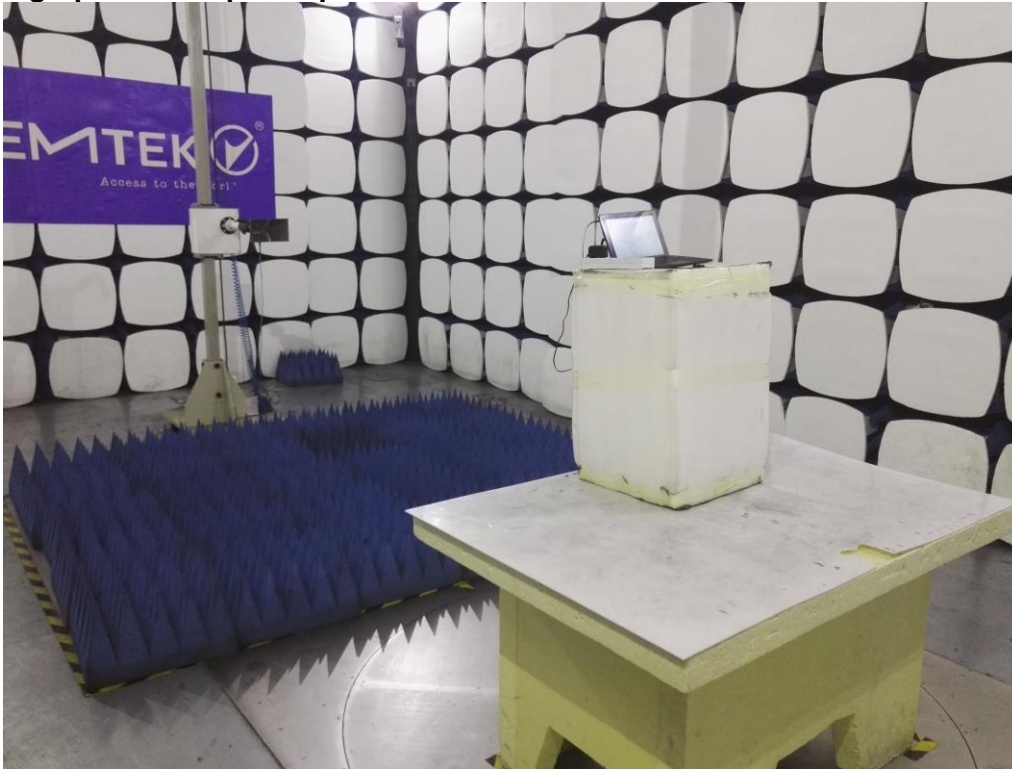
Photograph 4: Set-up for Spurious Emissions for 18 - 26.5GHz
