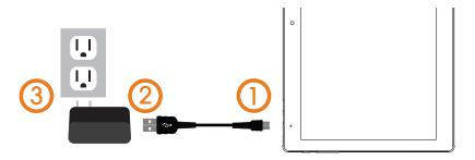
AC adapter (2), and plug the AC adapter into a wall outlet (3). If the tablet is on, the battery icon will pulse, showing that it is being charged. It is fully charged when an icon of a full battery is displayed on the screen. A complete battery charge will take approximately 5 hours. It is normal for the tablet to be warm to the touch as it is being charged.
