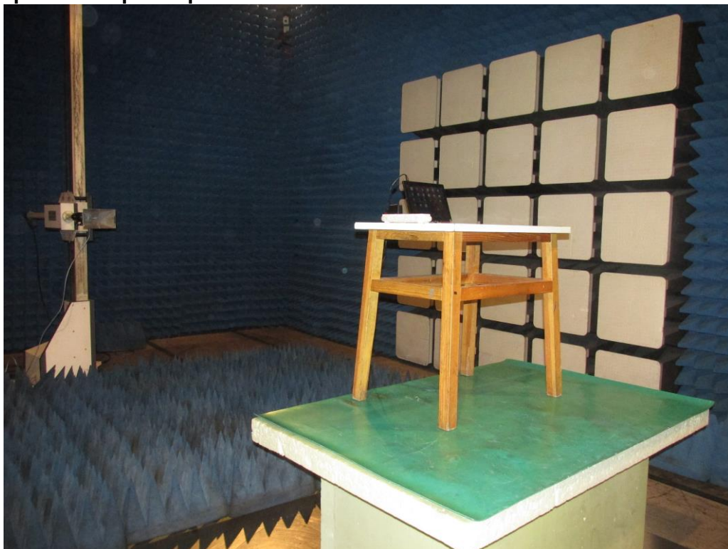
Photograph 4: Set-up for Spurious Emissions for 1 - 18GHz
