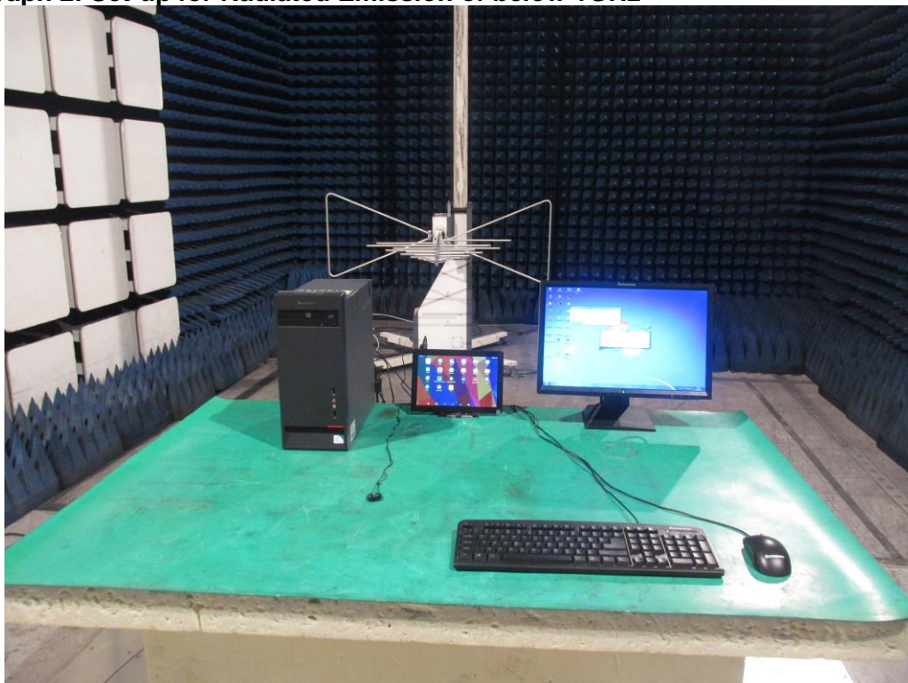
Photograph 2: Set-up for Radiated Emission of below 1GHz
