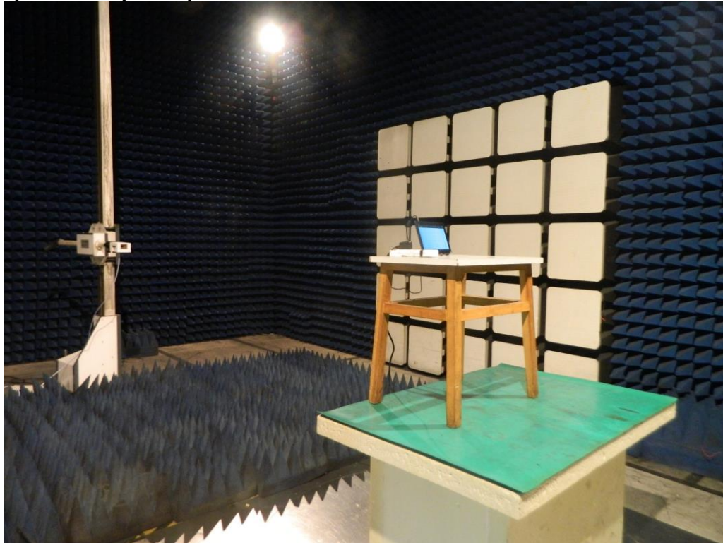
Photograph 5: Set-up for Spurious Emissions for 18 - 40GHz
