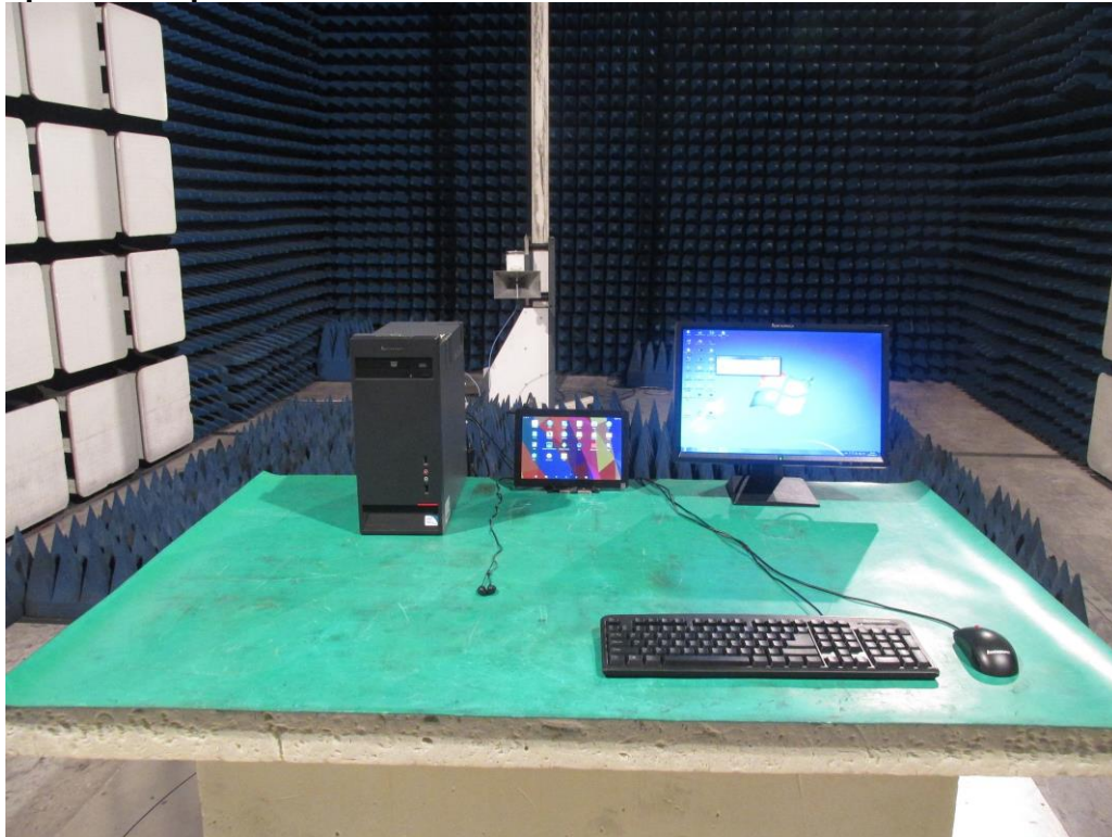
Photograph 3: Set-up for Radiated Emission of 1 - 18GHz
