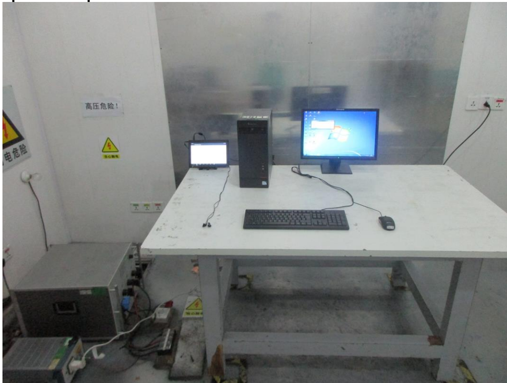
Photograph 2: Set-up for Radiated Emission of below 1GHz
