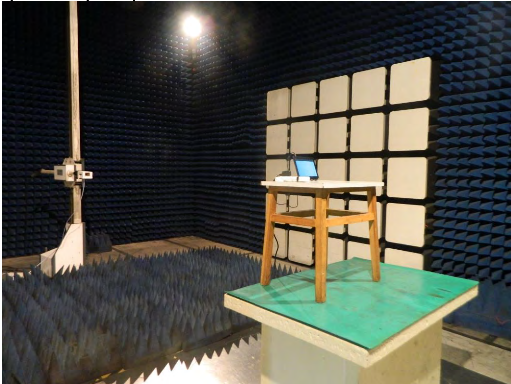
Photograph 5: Set-up for Spurious Emissions for 18 - 40GHz
