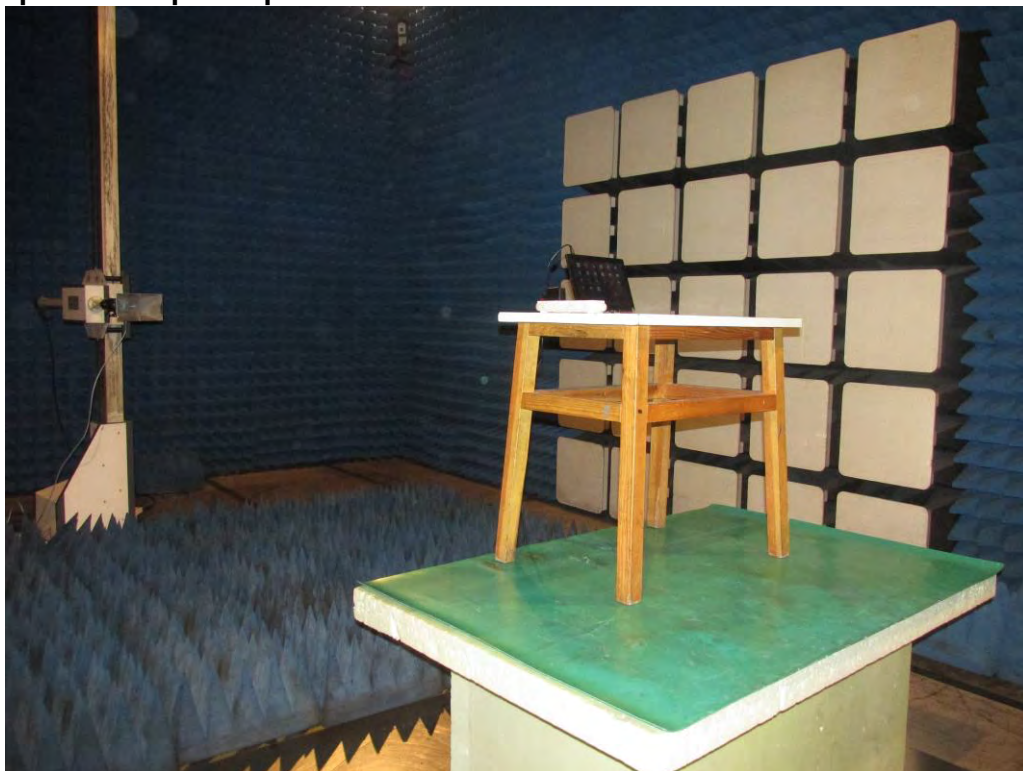
Photograph 4: Set-up for Spurious Emissions for 1 - 18GHz
