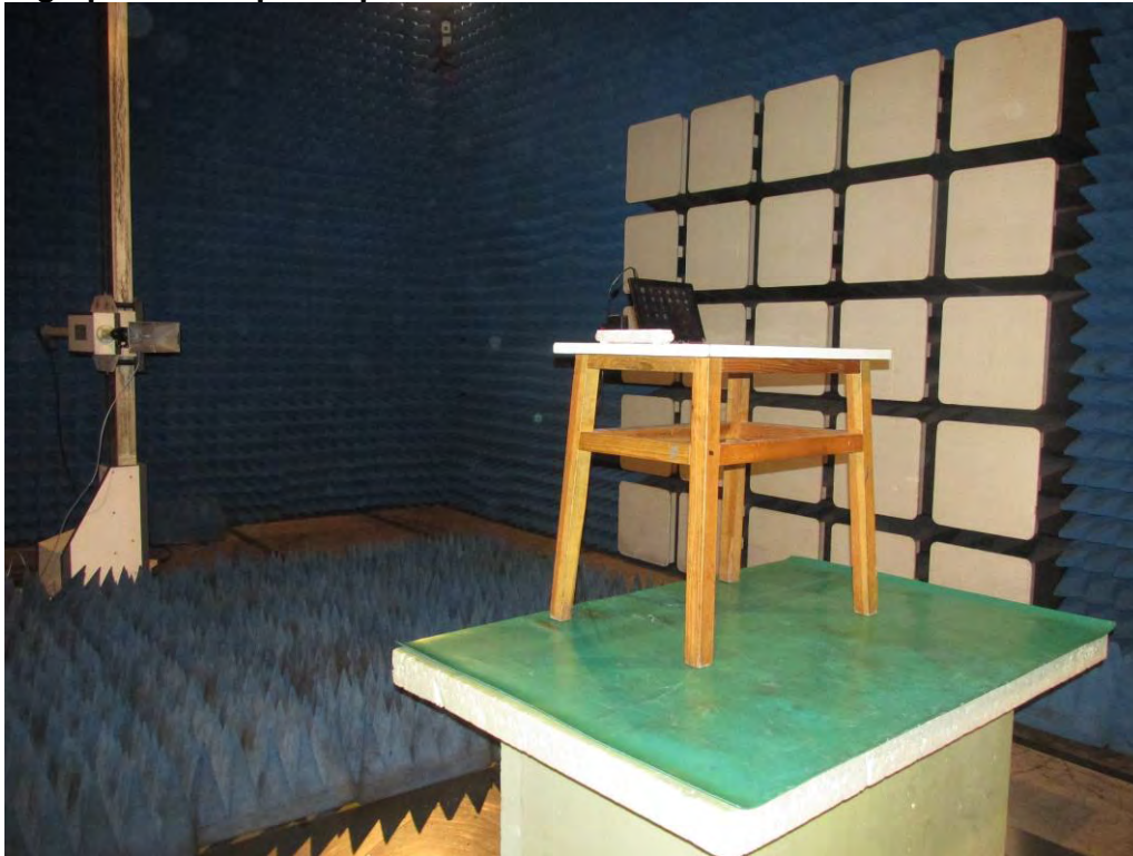
Photograph 4: Set-up for Spurious Emissions for 18 - 26.5GHz
