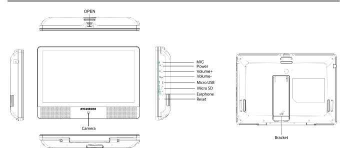
**OPEN(\nabla)**: Press it to open the unit and put the disc on the loading tray.
