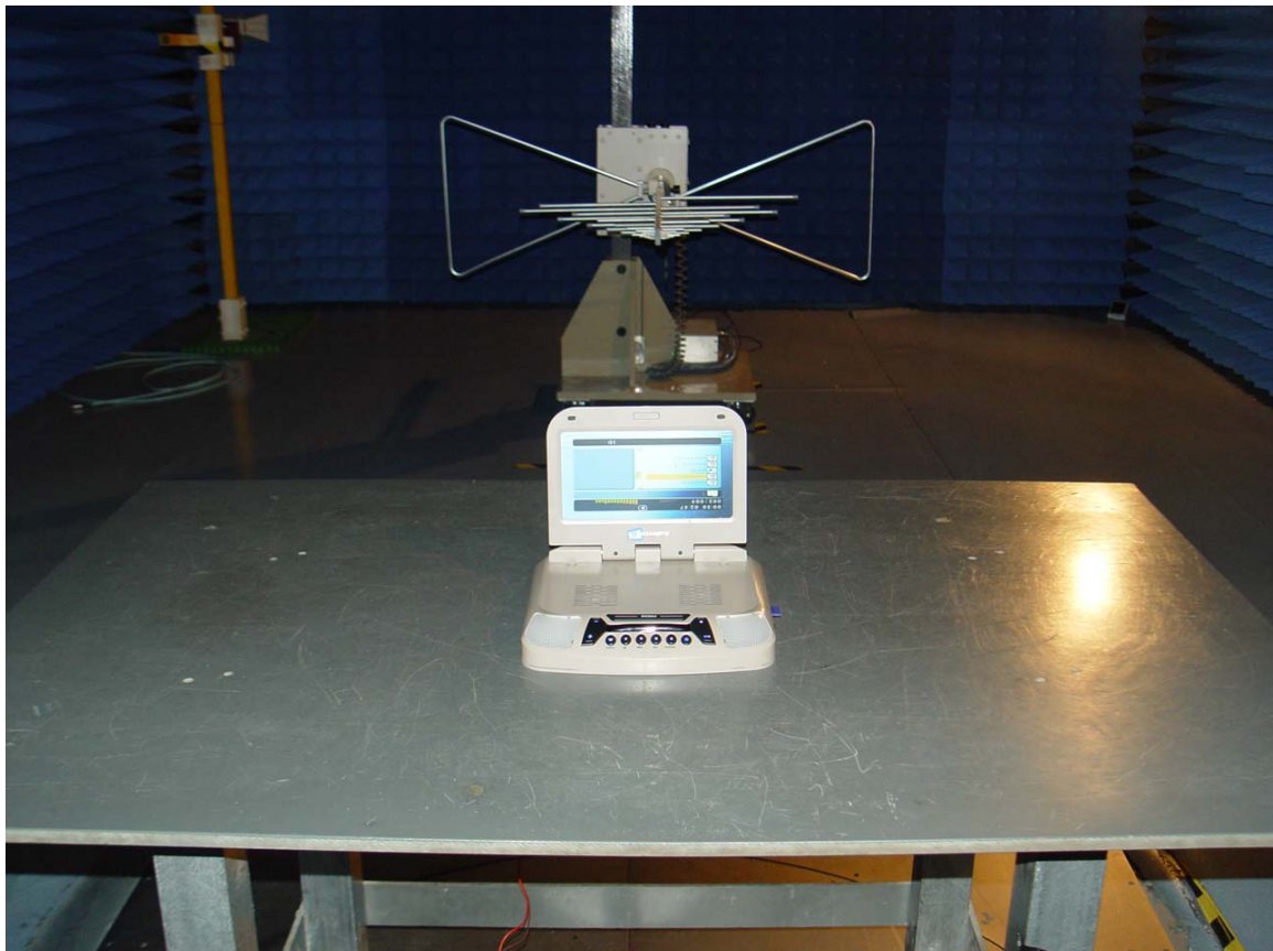
Radiated emissions test: TX with SD card
