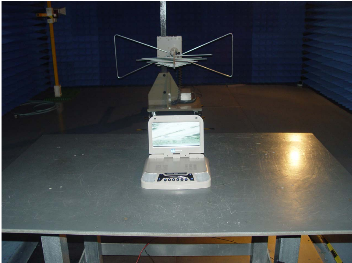
Radiated emissions test: TX with DVD
