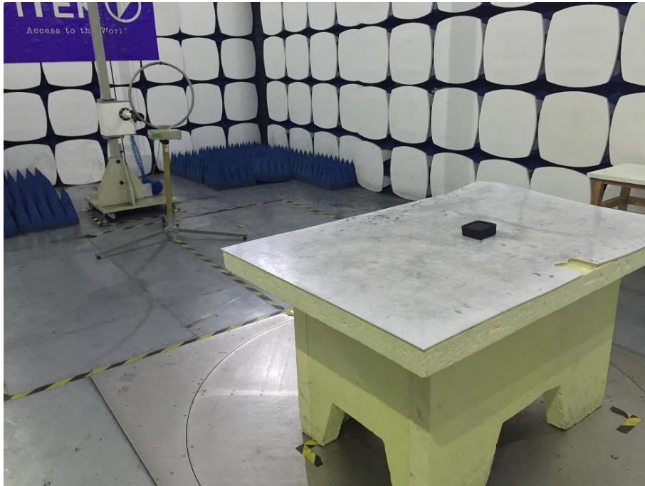
Photograph 1: Set-up for Radiated Spurious Emission (9kHz ~ 30MHz)
