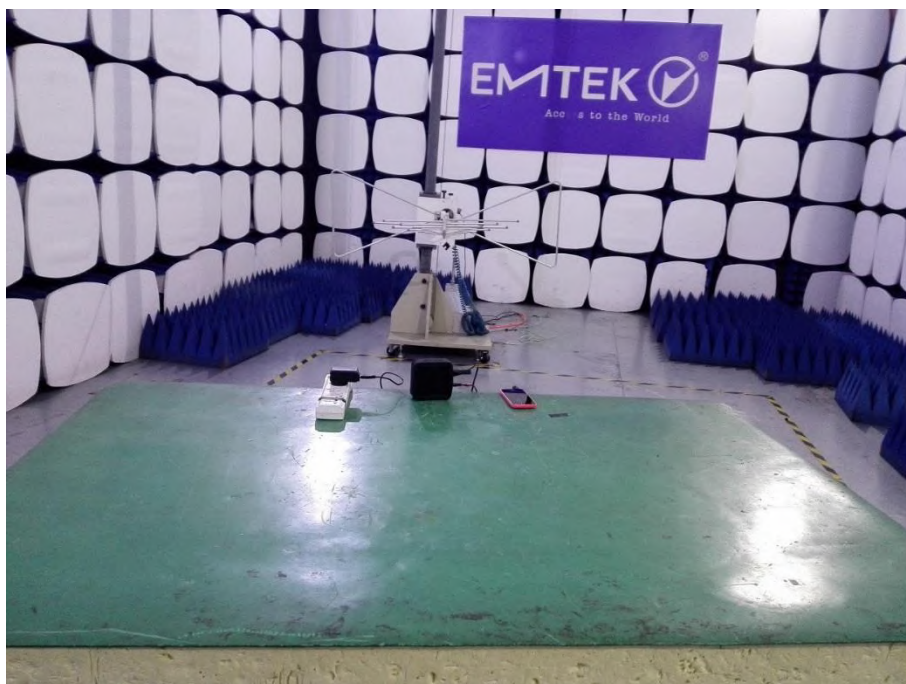
Photograph 6: Set-up for Radiated Emission (30MHz ~ 1GHz)
