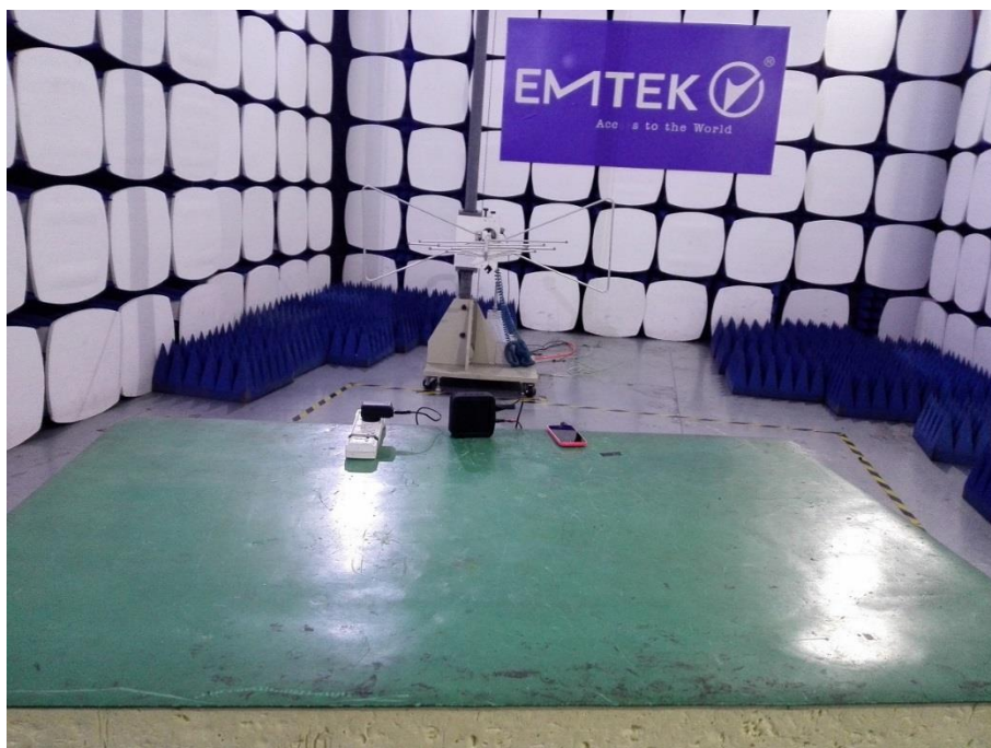
Photograph 6: Set-up for Radiated Emission (30MHz ~ 1GHz)
