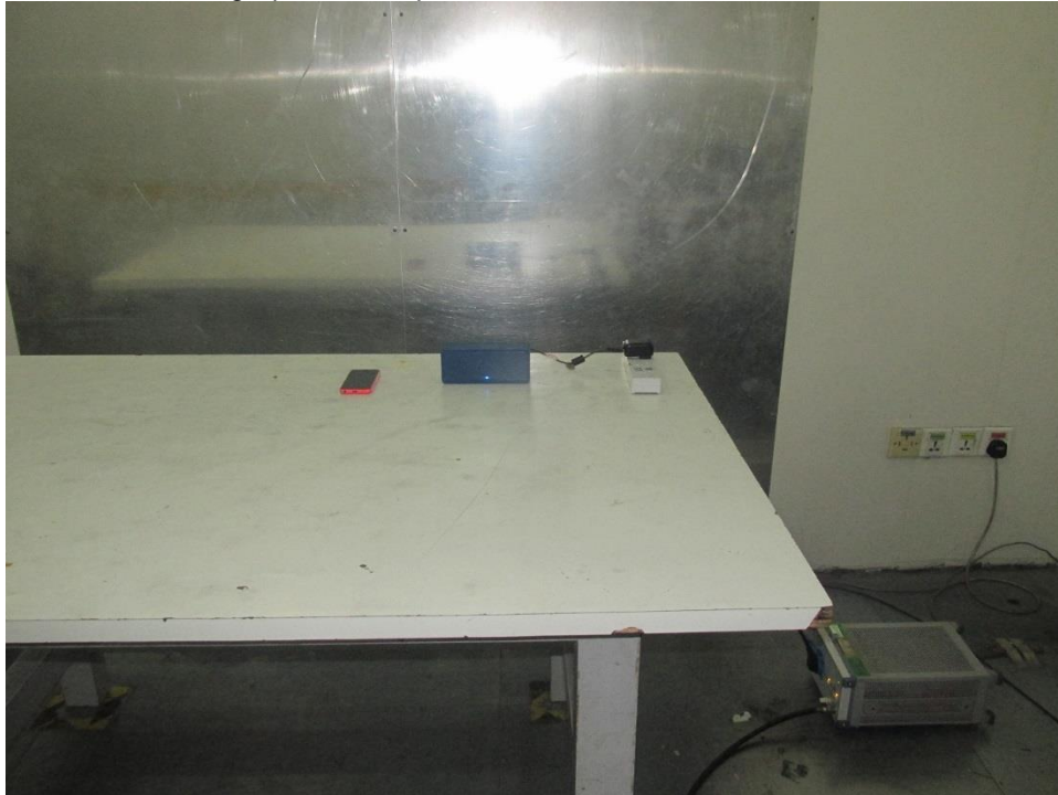
Photograph 5: Set-up for Conducted Emission on AC Mains
