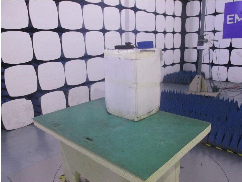
Photograph 4: Set-up for Radiated Spurious Emission above 18GHz
