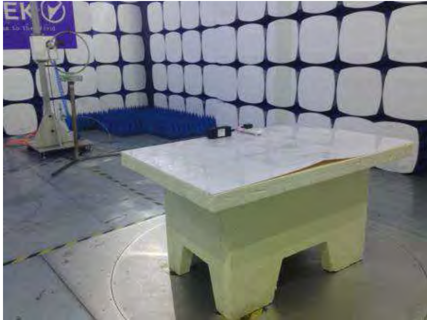
Photograph 2: Set-up for Radiated Spurious Emissions (30MHz-1GHz)
