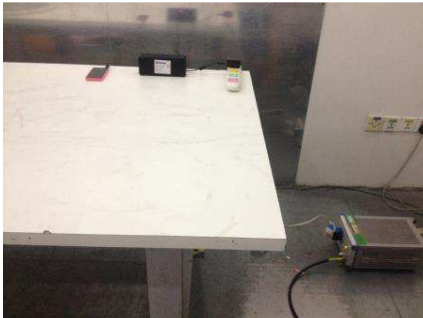
Photograph 4: Set-up for Conducted Emissions
