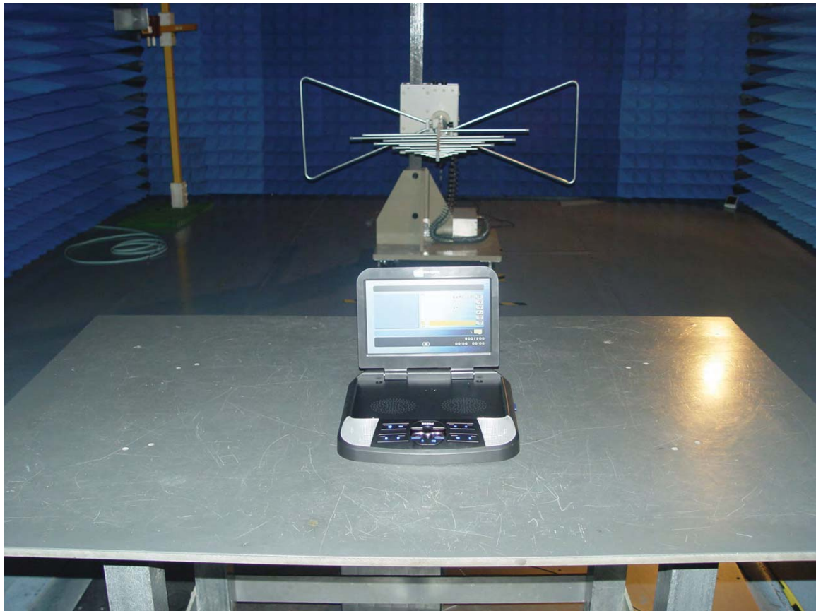
Radiated emissions test: TX with SD card
