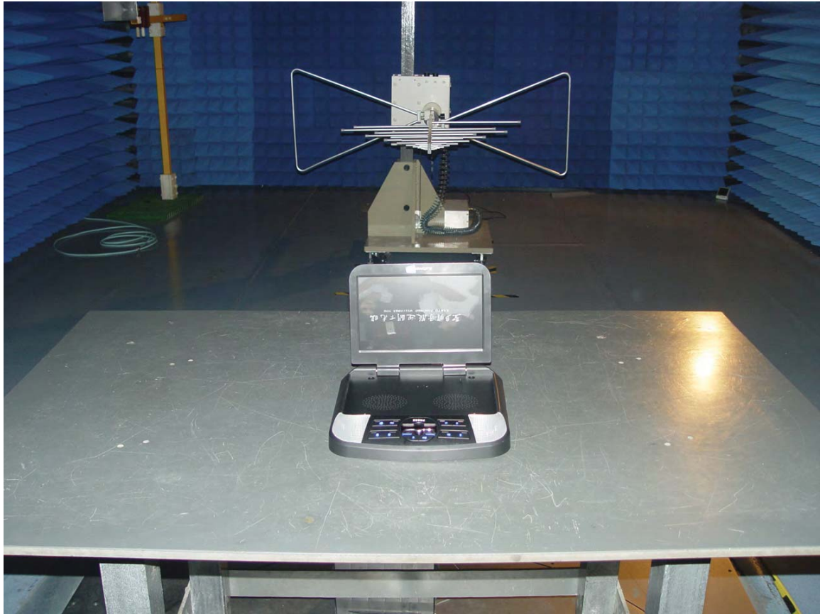
Radiated emissions test: TX with DVD
