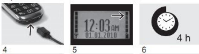
4. Connect charger cable to the socket on the bottom of the handset.
