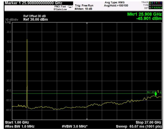
Channel: BOTTOM, Modulation: 256QAM, BW=15MHz, Range: 1GHz - 27GHz
