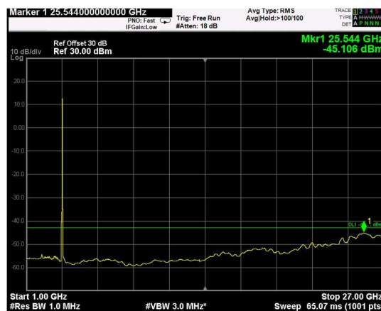
Channel: TOP, Modulation: 16QAM, BW=15MHz, Range: 1GHz - 27GHz
