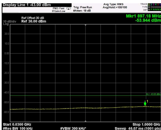
Channel: MIDDLE, Modulation: 16QAM, BW=20MHz, Range: 30MHz - 1GHz
