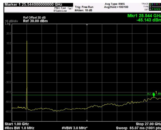
Channel: TOP, Modulation: QPSK, BW=20MHz, Range: 1GHz - 27GHz
