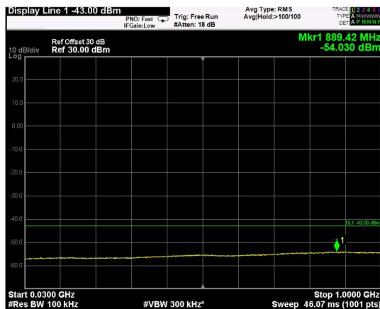
Channel: MIDDLE, Modulation: 64QAM, BW=20MHz, Range: 30MHz - 1GHz
