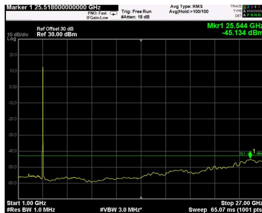
Channel: BOTTOM, Modulation: 256QAM, BW=20MHz, Range: 1GHz - 27GHz
