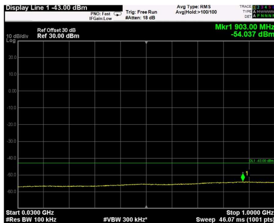
Channel: MIDDLE, Modulation: 256QAM, BW=20MHz, Range: 30MHz - 1GHz
