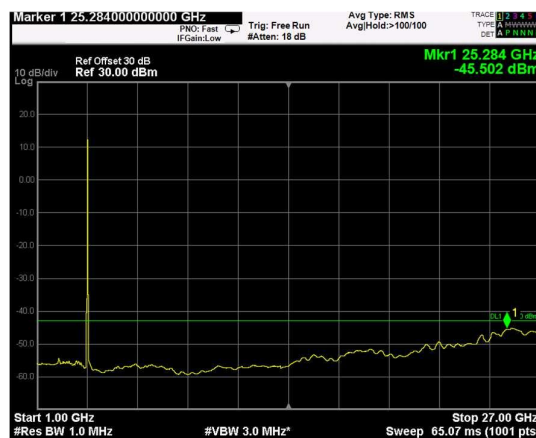
Channel: MIDDLE, Modulation: 16QAM, BW=15MHz, Range: 1GHz - 27GHz
