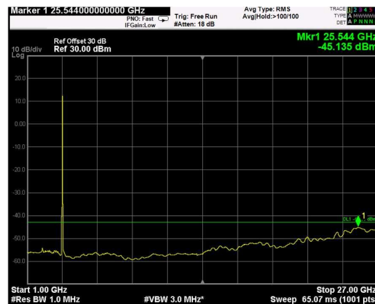
Channel: MIDDLE, Modulation: 64QAM, BW=20MHz, Range: 1GHz - 27GHz
