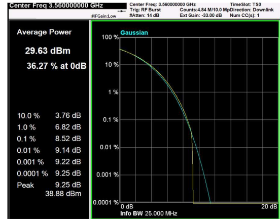
Channel: BOTTOM, Modulation: 16QAM, BW=20MHz, CCDF
