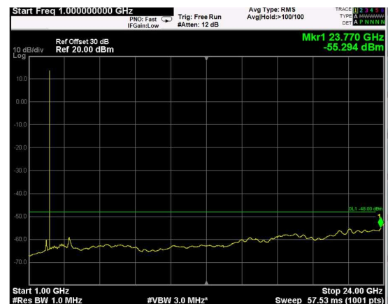
Channel: TOP, Modulation: 256QAM, BW=5MHz, Range: Upper
