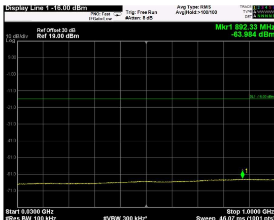
Channel: TOP, Modulation: 64QAM, BW=20MHz, Range: Lower
