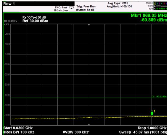
Channel: BOTTOM, Modulation: 16QAM, BW=15MHz, Range: 30MHz - 1GHz
