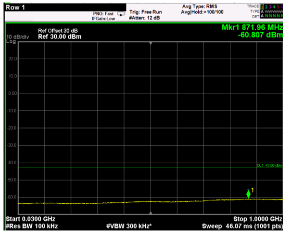
Channel: TOP, Modulation: 64QAM, BW=15MHz, Range: 30MHz - 1GHz
