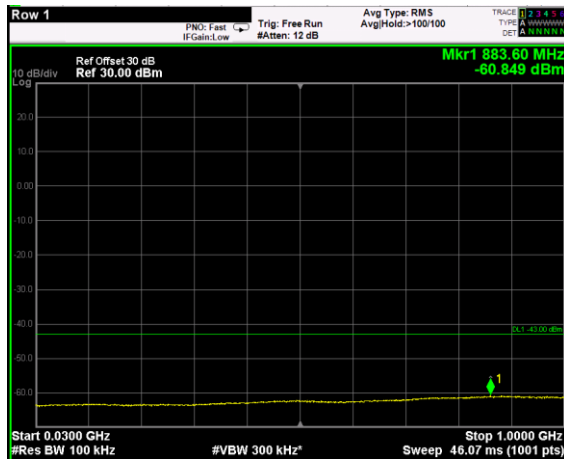
Channel: MIDDLE, Modulation: 16QAM, BW=15MHz, Range: 30MHz - 1GHz
