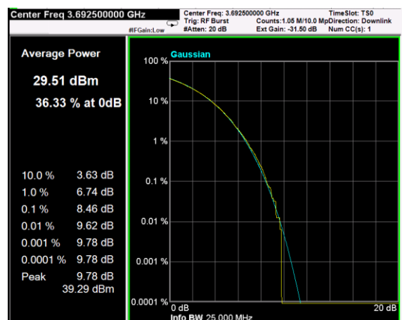
Channel: TOP, Modulation: 16QAM, BW=15MHz, CCDF
