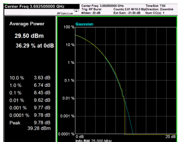
Channel: TOP, Modulation: 64QAM, BW=15MHz, CCDF
