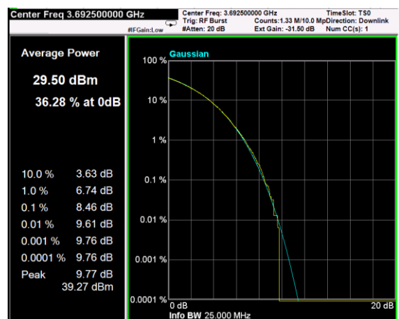
Channel: TOP, Modulation: QPSK, BW=15MHz, CCDF
