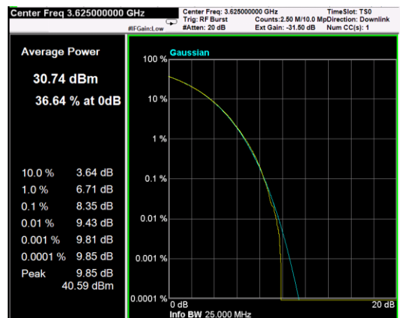
Channel: MIDDLE, Modulation: QPSK, BW=15MHz, CCDF
