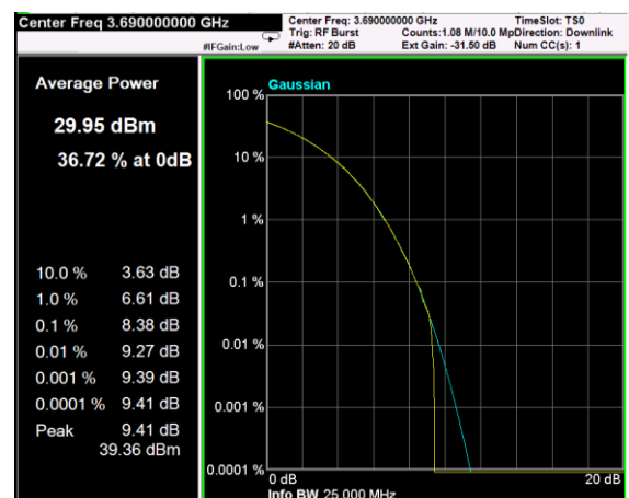
Channel: TOP, Modulation: 16QAM, BW=20MHz, CCDF
