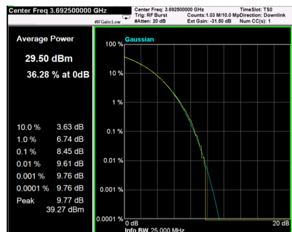
Channel: TOP, Modulation: 256QAM, BW=15MHz, CCDF
