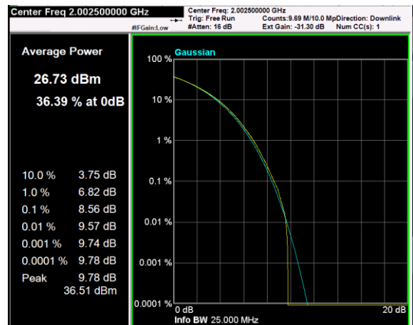
Channel: BOTTOM, Modulation: QPSK, BW=15MHz, CCDF
