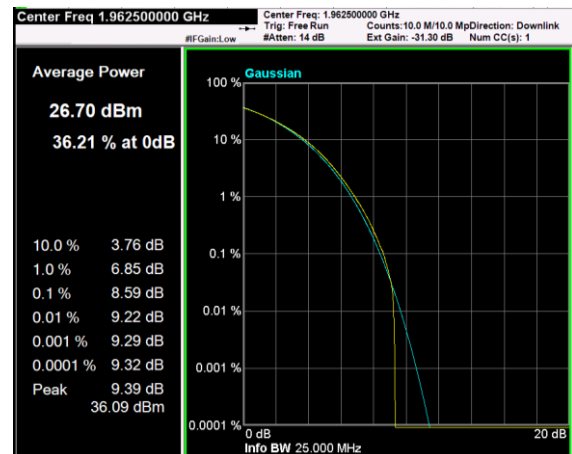
Channel: MIDDLE, Modulation: 64QAM, BW=20MHz, CCDF
