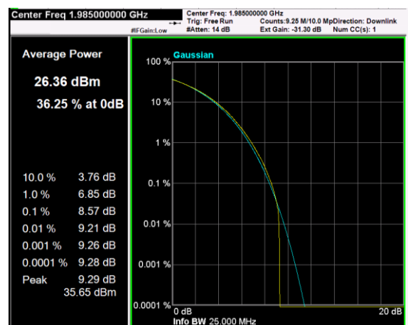
Channel: TOP, Modulation: 256QAM, BW=20MHz, CCDF
