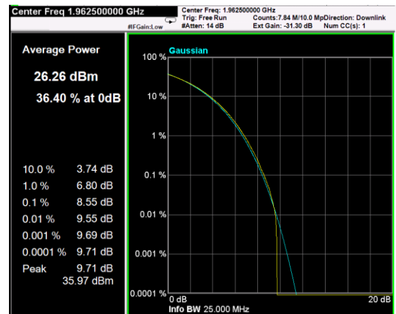
Channel: MIDDLE, Modulation: 16QAM, BW=15MHz, CCDF
