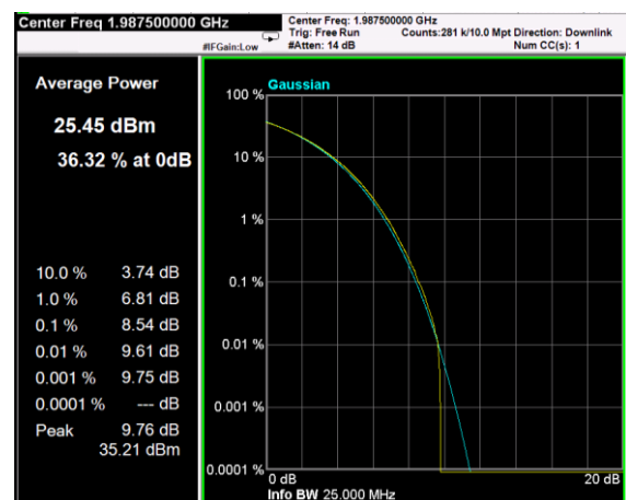
Channel: TOP, Modulation: 256QAM, BW=15MHz, CCDF
