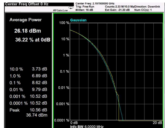
Channel: TOP, Modulation: 256QAM, BW=5MHz, CCDF
