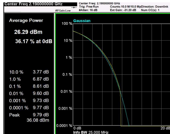
Channel: MIDDLE, Modulation: 256QAM, BW=15MHz, CCDF
