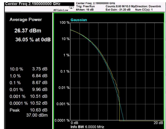
Channel: MIDDLE, Modulation: 256QAM, BW=5MHz, CCDF
