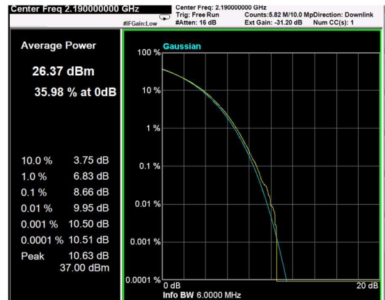
Channel: MIDDLE, Modulation: 64QAM, BW=5MHz, CCDF
