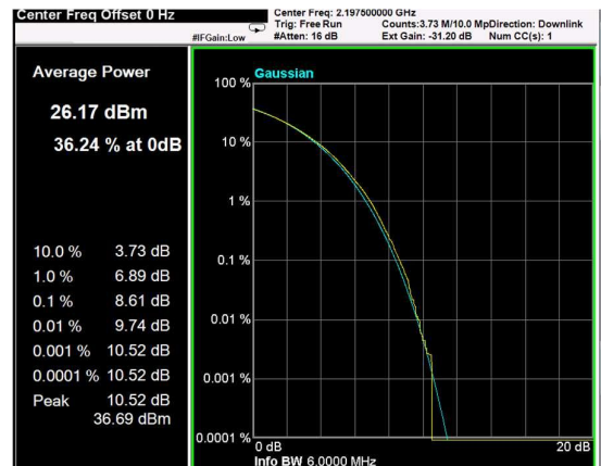
Channel: TOP, Modulation: 64QAM, BW=5MHz, CCDF
