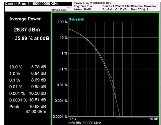
Channel: MIDDLE, Modulation: 16QAM, BW=5MHz, CCDF
