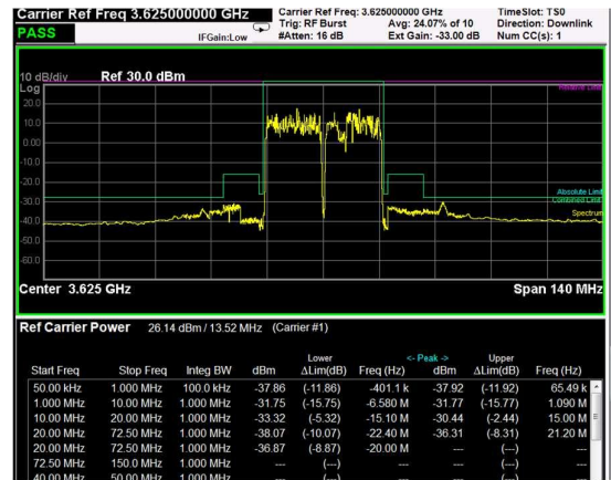
Middle Band Edge, 2 Carrier, Modulation: 16QAM, BW=15MHz
