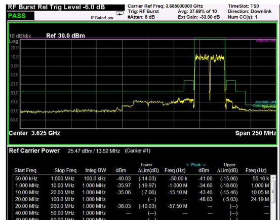
High Band Edge, 2 Carrier, Modulation: QPSK, BW=15MHz
