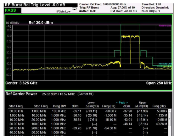
High Band Edge, 2 Carrier, Modulation: 16QAM, BW=15MHz
