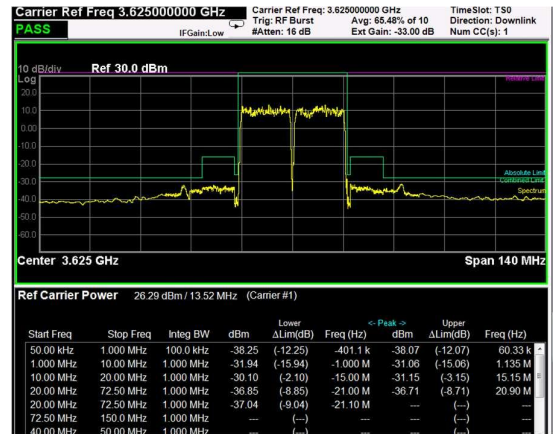
Middle Band Edge, 2 Carrier, Modulation: QPSK, BW=15MHz
