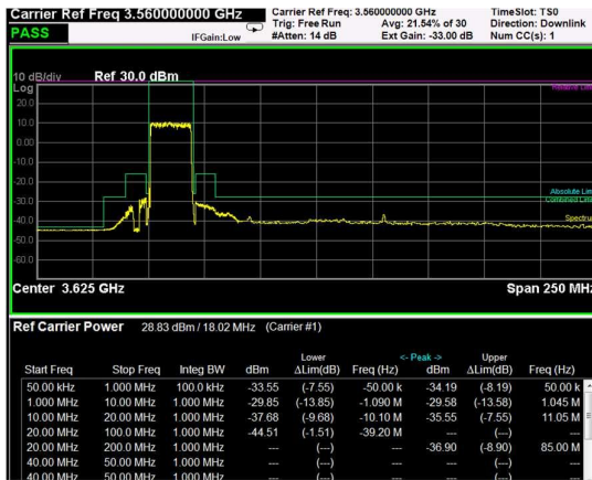
Low Band Edge, 1 Carrier, Modulation: 16QAM, BW=20MHz
