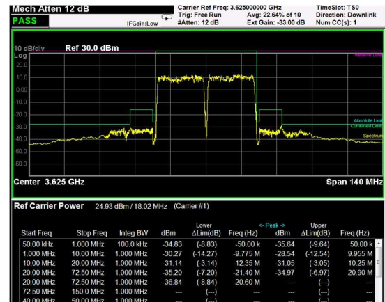
Middle Band Edge, 2 Carrier, Modulation: 16QAM, BW=20MHz
