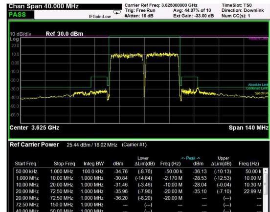
Middle Band Edge, 2 Carrier, Modulation: 64QAM, BW=20MHz
