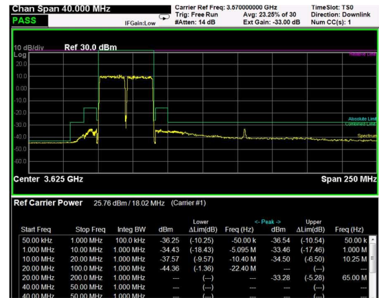
Low Band Edge, 2 Carrier, Modulation: 64QAM, BW=20MHz
