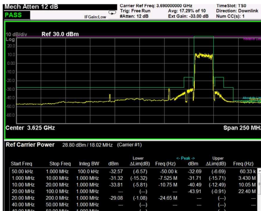
High Band Edge, 1 Carrier, Modulation: 16QAM, BW=20MHz
