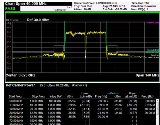
Middle Band Edge, 2 Carrier, Modulation: 256QAM, BW=20MHz
