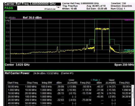
High Band Edge, 2 Carrier, Modulation: 256QAM, BW=15MHz
