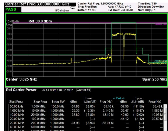
High Band Edge, 2 Carrier, Modulation: 16QAM, BW=20MHz
