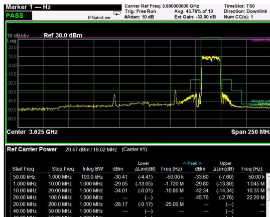
High Band Edge, 1 Carrier, Modulation: QPSK, BW=20MHz
