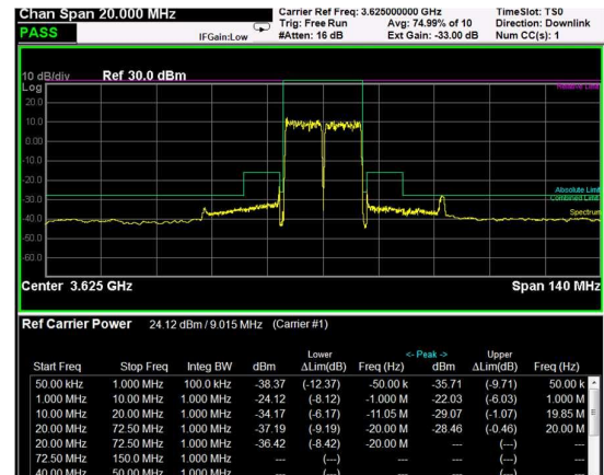
Middle Band Edge, 2 Carrier, Modulation: 64QAM, BW=10MHz
