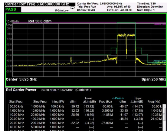
High Band Edge, 2 Carrier, Modulation: 64QAM, BW=15MHz
