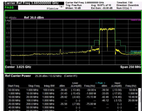
High Band Edge, 2 Carrier, Modulation: QPSK, BW=15MHz
