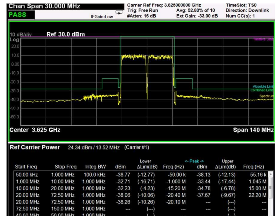
Middle Band Edge, 2 Carrier, Modulation: 16QAM, BW=15MHz
