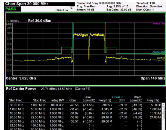
Middle Band Edge, 2 Carrier, Modulation: 64QAM, BW=15MHz
