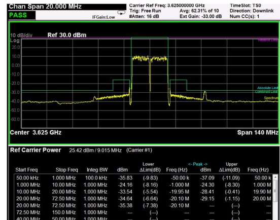
Middle Band Edge, 2 Carrier, Modulation: 16QAM, BW=10MHz
