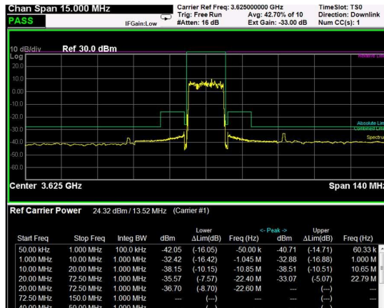
Middle Band Edge, 1 Carrier, Modulation: QPSK, BW=15MHz
