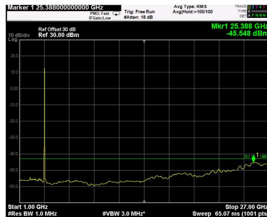
Channel: TOP, Modulation: QPSK, BW=15MHz, Range: 1GHz - 27GHz
