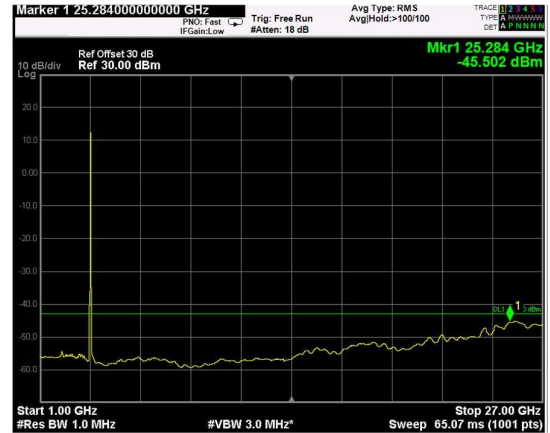
Channel: MIDDLE, Modulation: 16QAM, BW=15MHz, Range: 1GHz - 27GHz
