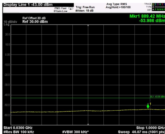
Channel: TOP, Modulation: 256QAM, BW=15MHz, Range: 30MHz - 1GHz
