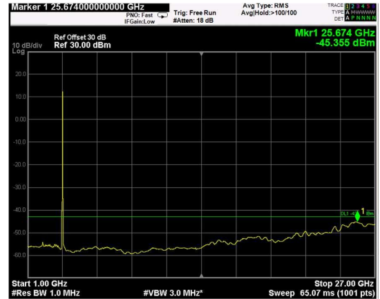
Channel: BOTTOM, Modulation: 16QAM, BW=20MHz, Range: 1GHz - 27GHz
