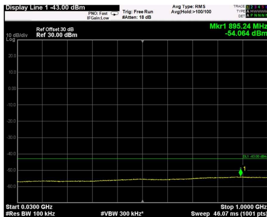
Channel: MIDDLE, Modulation: QPSK, BW=20MHz, Range: 30MHz - 1GHz
