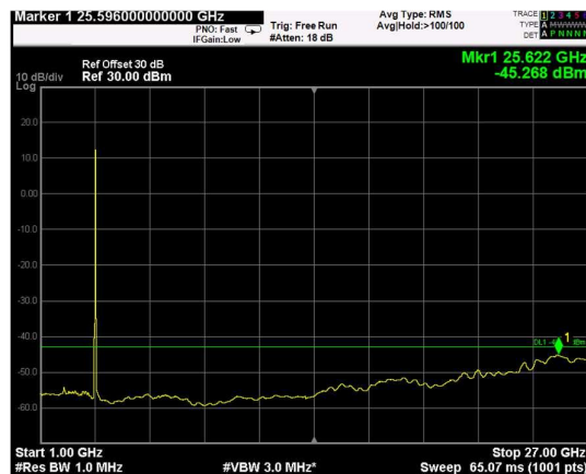
Channel: BOTTOM, Modulation: 64QAM, BW=20MHz, Range: 1GHz - 27GHz
