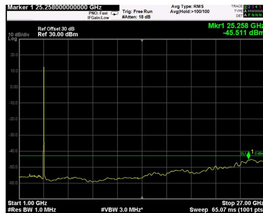
Channel: TOP, Modulation: 256QAM, BW=15MHz, Range: 1GHz - 27GHz
