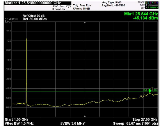
Channel: BOTTOM, Modulation: 256QAM, BW=20MHz, Range: 1GHz - 27GHz
