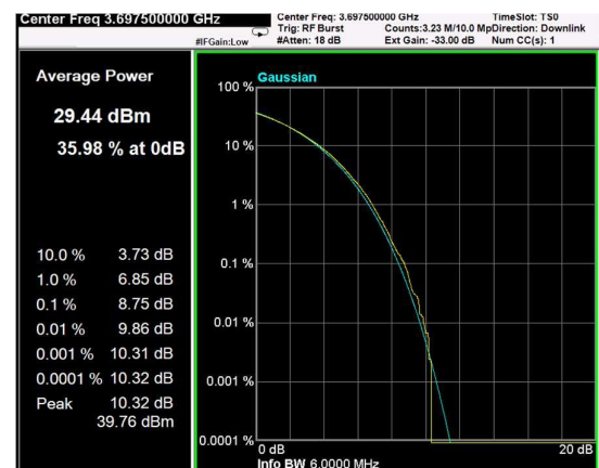
Channel: TOP, Modulation: 16QAM, BW=5MHz, CCDF
