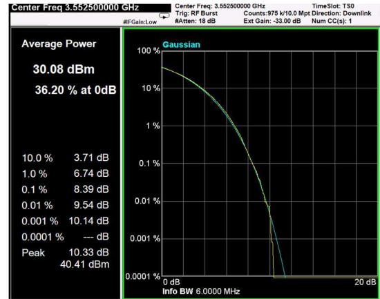
Channel: BOTTOM, Modulation: 64QAM, BW=5MHz, CCDF
