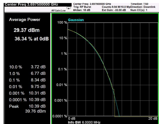
Channel: TOP, Modulation: 64QAM, BW=5MHz, CCDF
