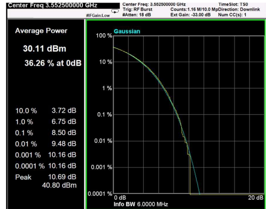
Channel: BOTTOM, Modulation: QPSK, BW=5MHz, CCDF
