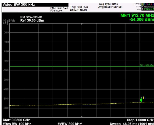
Channel: TOP, Modulation: 256QAM, BW=5MHz, Range: Lower
