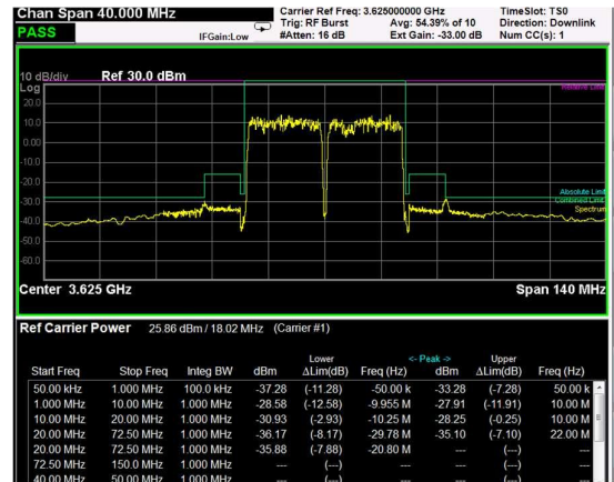
Middle Band Edge, 2 Carrier, Modulation: QPSK, BW=20MHz
