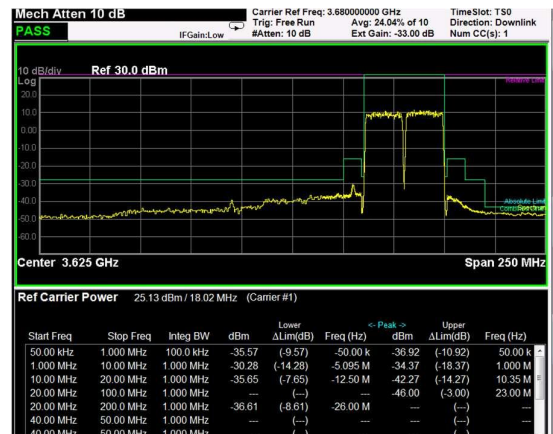
High Band Edge, 2 Carrier, Modulation: QPSK, BW=20MHz
