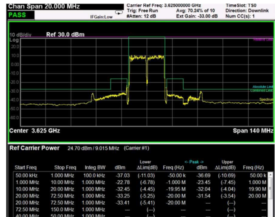
Middle Band Edge, 2 Carrier, Modulation: 16QAM, BW=10MHz
