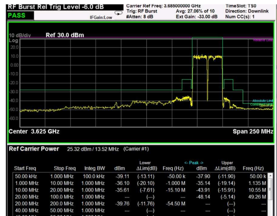
High Band Edge, 2 Carrier, Modulation: 16QAM, BW=15MHz
