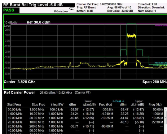
High Band Edge, 1 Carrier, Modulation: 64QAM, BW=15MHz
