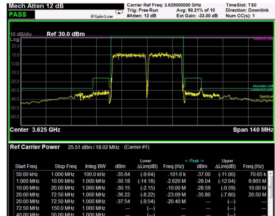
Middle Band Edge, 2 Carrier, Modulation: QPSK, BW=20MHz
