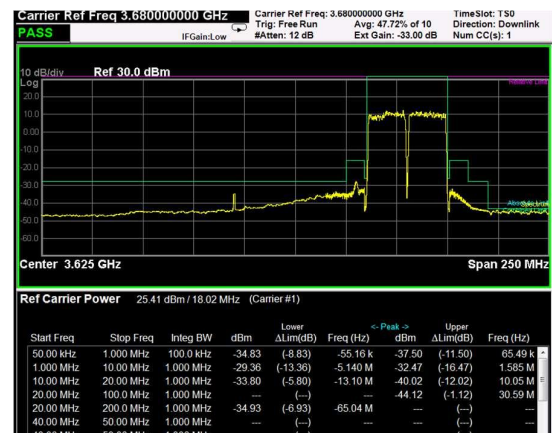
High Band Edge, 2 Carrier, Modulation: 16QAM, BW=20MHz
