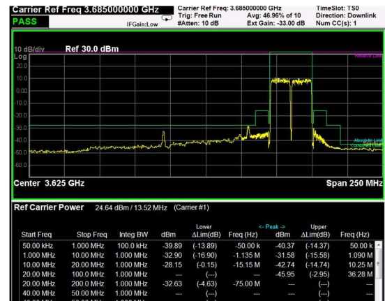
High Band Edge, 2 Carrier, Modulation: 256QAM, BW=15MHz
