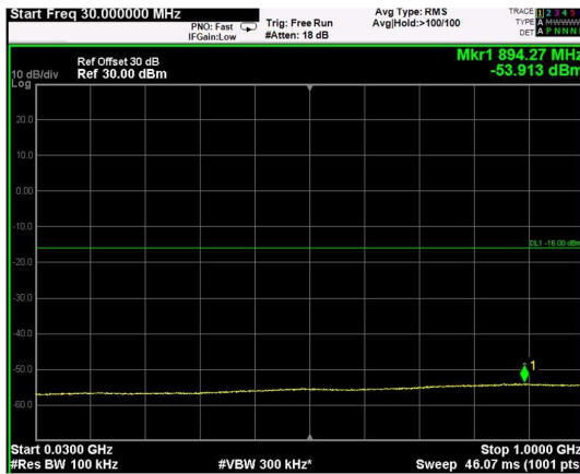
Channel: MIDDLE, Modulation: 256QAM, BW=5MHz, Range: Lower
