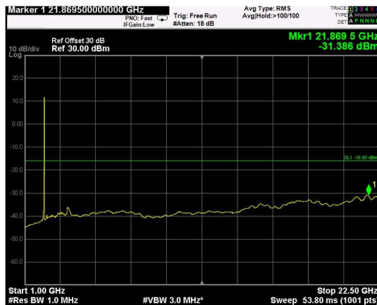
Channel: MIDDLE, Modulation: QPSK, BW=10MHz, Range: Upper
