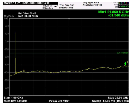
Channel: BOTTOM, Modulation: 16QAM, BW=15MHz, Range: Upper
