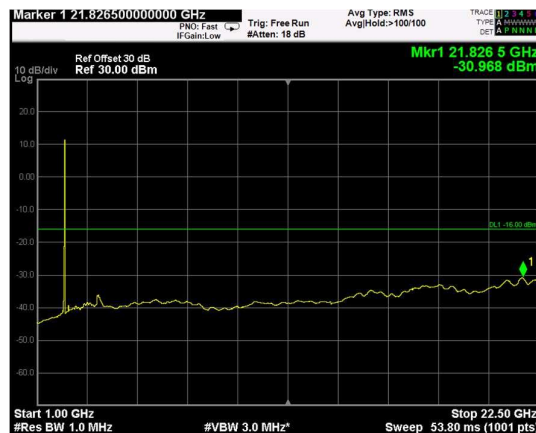
Channel: BOTTOM, Modulation: 64QAM, BW=10MHz, Range: Upper
