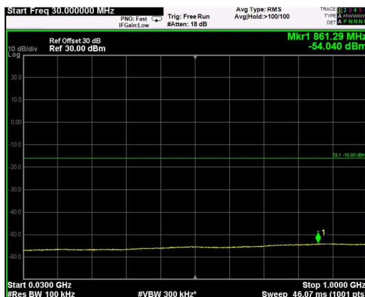
Channel: TOP, Modulation: 64QAM, BW=15MHz, Range: Lower
