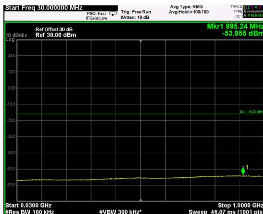
Channel: TOP, Modulation: 256QAM, BW=15MHz, Range: Lower
