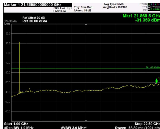
Channel: TOP, Modulation: 64QAM, BW=10MHz, Range: Upper
