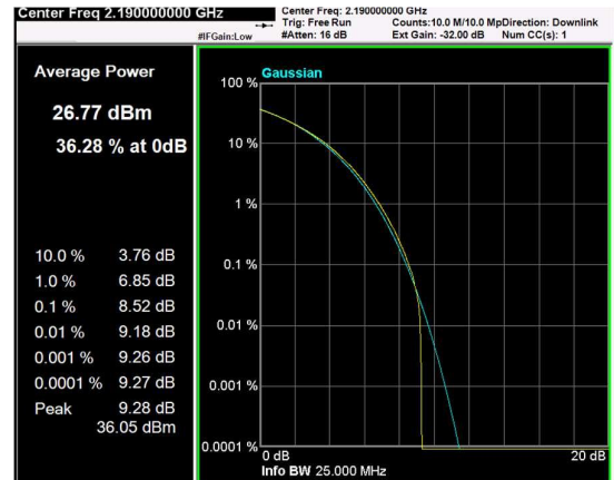
Channel: MIDDLE, Modulation: 256QAM, BW=10MHz, CCDF
