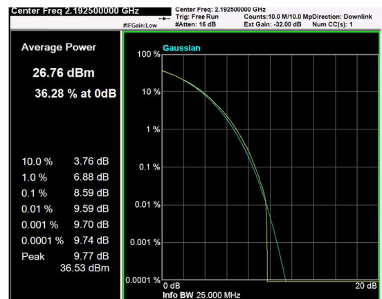
Channel: TOP, Modulation: 256QAM, BW=15MHz, CCDF
