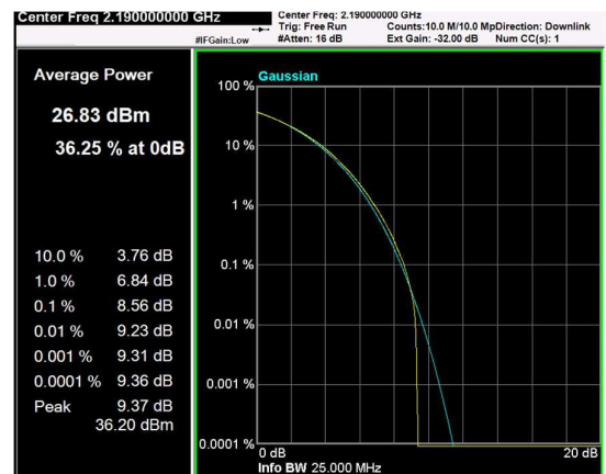
Channel: MIDDLE, Modulation: 64QAM, BW=20MHz, CCDF
