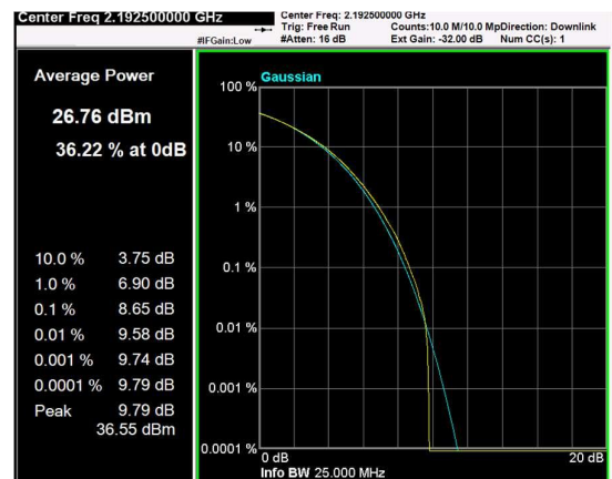
Channel: TOP, Modulation: 16QAM, BW=15MHz, CCDF
