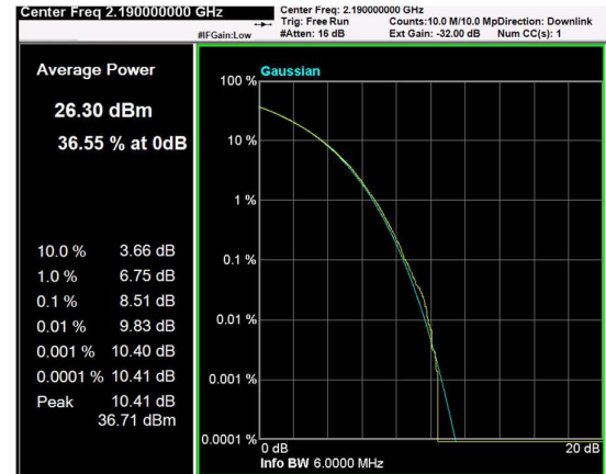
Channel: MIDDLE, Modulation: QPSK, BW=5MHz, CCDF
