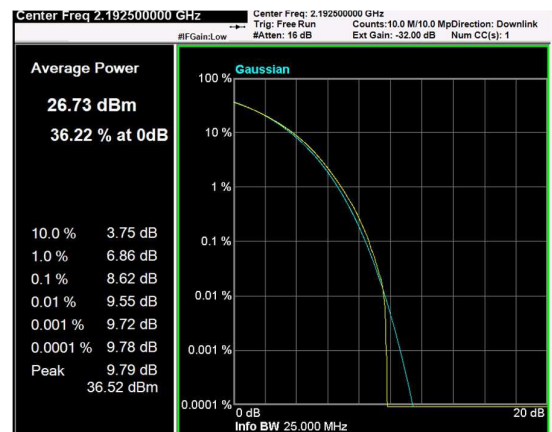
Channel: TOP, Modulation: QPSK, BW=15MHz, CCDF
