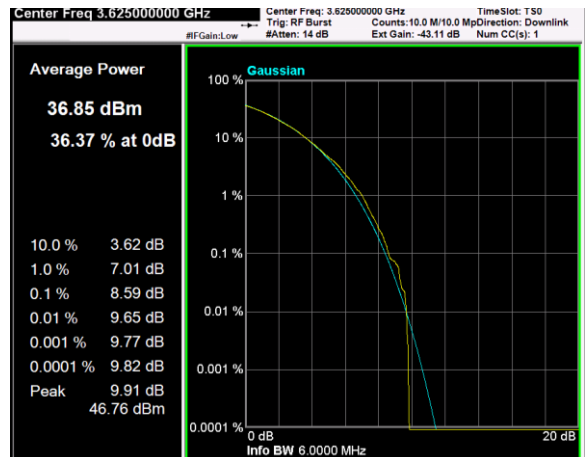
Channel: MIDDLE, Modulation: QPSK, BW=5MHz, CCDF
