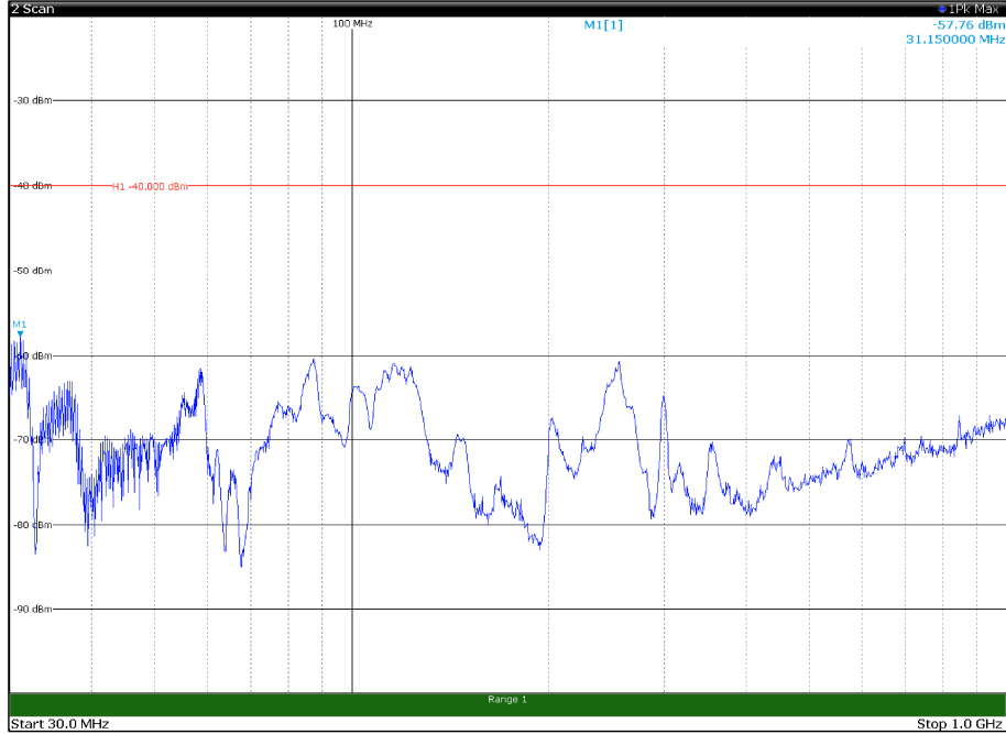
Channel: TOP, Modulation: QPSK, BW=10MHz, Range: 30MHz- 1GHz, Polarization: Vertical
