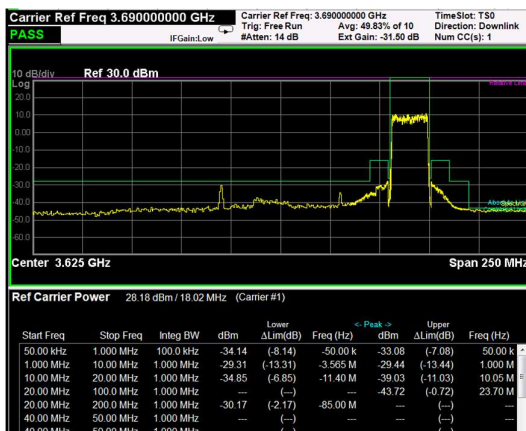
High Band Edge, 1 Carrier, Modulation: 16QAM, BW=20MHz
