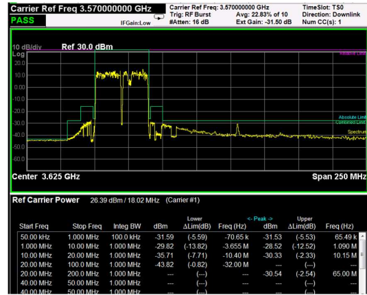
Low Band Edge, 2 Carrier, Modulation: 16QAM, BW=20MHz
