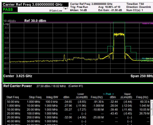
High Band Edge, 1 Carrier, Modulation: 256QAM, BW=20MHz
