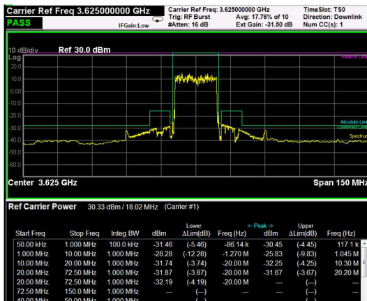
Middle Band Edge, 1 Carrier, Modulation: 16QAM, BW=20MHz
