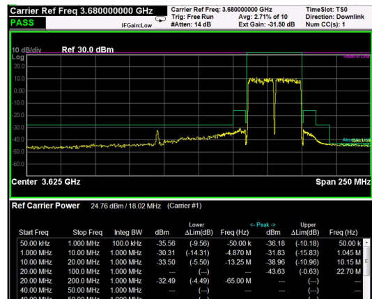
High Band Edge, 2 Carrier, Modulation: 256QAM, BW=20MHz
