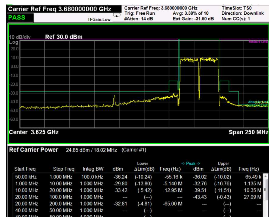
High Band Edge, 2 Carrier, Modulation: 16QAM, BW=20MHz
