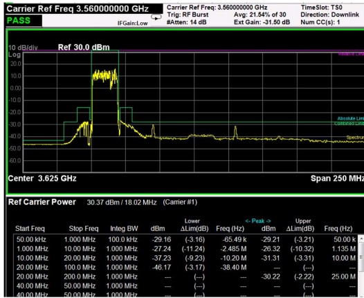
Low Band Edge, 1 Carrier, Modulation: 64QAM, BW=20MHz
