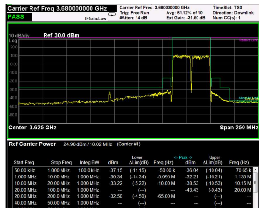
High Band Edge, 2 Carrier, Modulation: 64QAM, BW=20MHz
