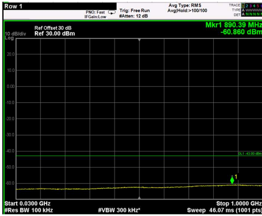
Channel: MIDDLE, Modulation: 256QAM, BW=15MHz, Range: 30MHz - 1GHz
