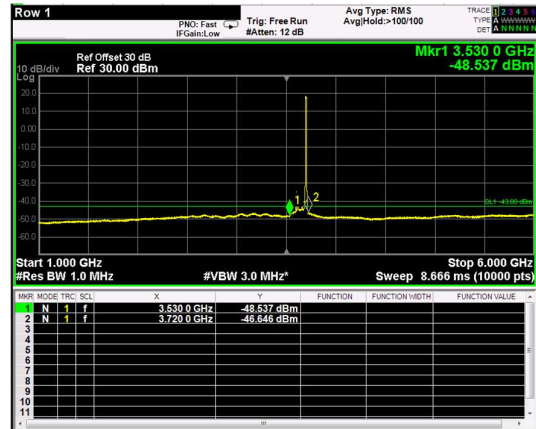
Channel: TOP, Modulation: QPSK, BW=10MHz, Range: 1GHz - 6GHz
