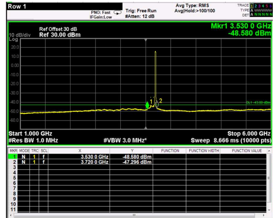
Channel: TOP, Modulation: 64QAM, BW=15MHz, Range: 1GHz - 6GHz
