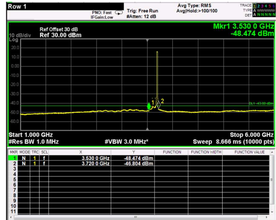
Channel: TOP, Modulation: 256QAM, BW=15MHz, Range: 1GHz - 6GHz
