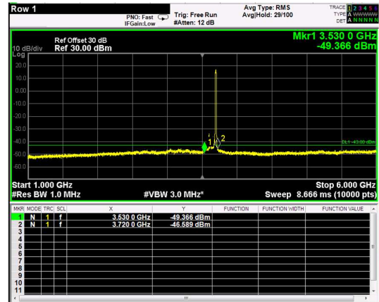
Channel: TOP, Modulation: QPSK, BW=15MHz, Range: 1GHz - 6GHz
