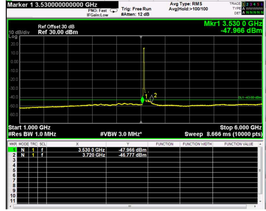
Channel: BOTTOM, Modulation: 64QAM, BW=20MHz, Range: 1GHz - 6GHz
