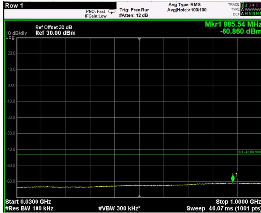
Channel: BOTTOM, Modulation: QPSK, BW=5MHz, Range: 30MHz - 1GHz
