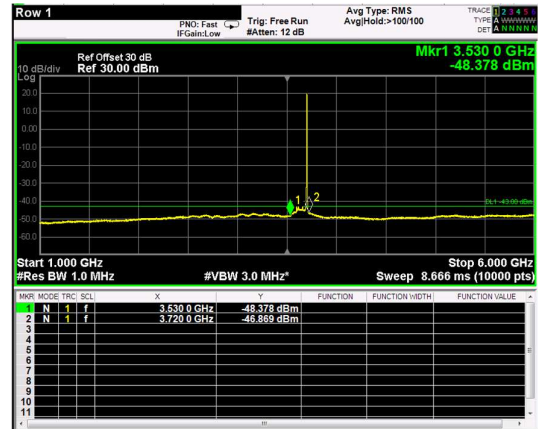
Channel: TOP, Modulation: 256QAM, BW=5MHz, Range: 1GHz - 6GHz
