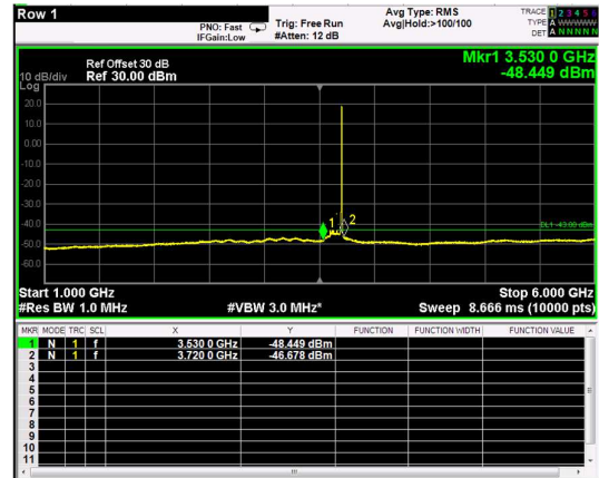
Channel: TOP, Modulation: QPSK, BW=5MHz, Range: 1GHz - 6GHz
