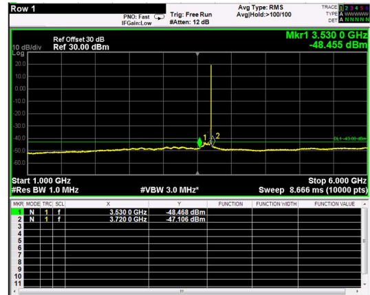
Channel: TOP, Modulation: 64QAM, BW=5MHz, Range: 1GHz - 6GHz
