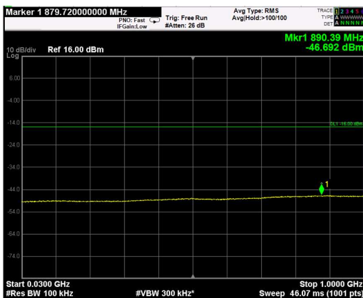
Channel: TOP, Modulation: 64QAM, BW=15MHz, Range: Lower
