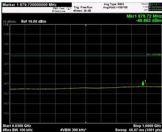
Channel: TOP, Modulation: 256QAM, BW=15MHz, Range: Lower
