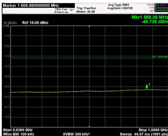
Channel: TOP, Modulation: 256QAM, BW=5MHz, Range: Lower
