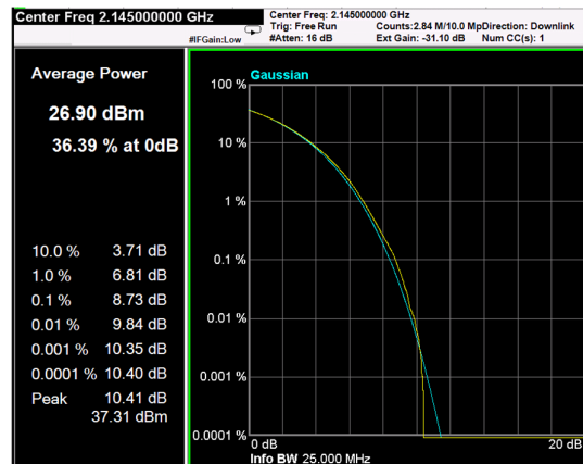
Channel: MIDDLE, Modulation: 256QAM, BW=5MHz, CCDF
