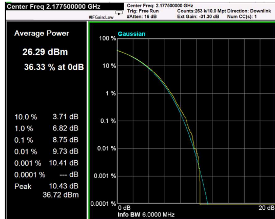
Channel: TOP, Modulation: QPSK, BW=5MHz, CCDF
