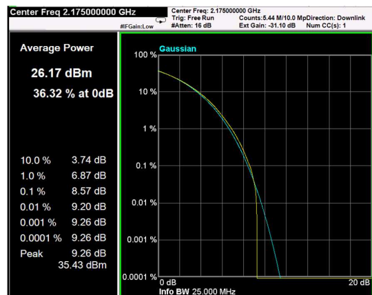
Channel: TOP, Modulation: 256QAM, BW=10MHz, CCDF
