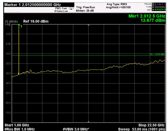
Channel: TOP, Modulation: 16QAM, BW=15MHz, Range: Upper
