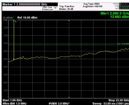
Channel: BOTTOM, Modulation: QPSK, BW=10MHz, Range: Upper
