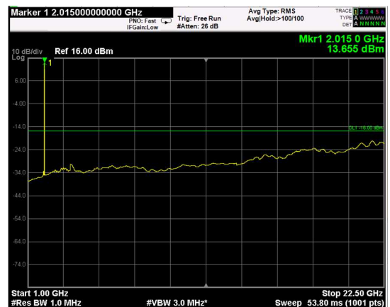
Channel: TOP, Modulation: 256QAM, BW=10MHz, Range: Upper
