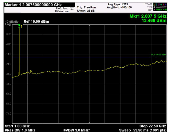
Channel: MIDDLE, Modulation: 16QAM, BW=20MHz, Range: Upper
