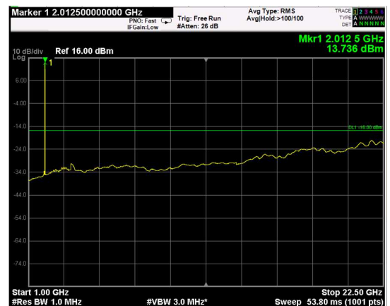
Channel: TOP, Modulation: 256QAM, BW=15MHz, Range: Upper
