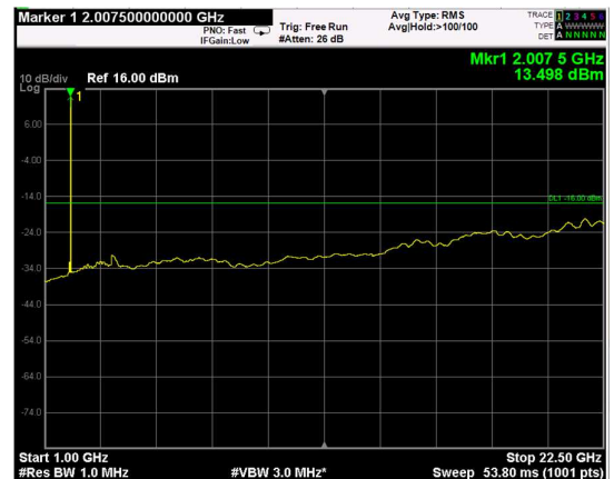
Channel: MIDDLE, Modulation: 256QAM, BW=15MHz, Range: Upper
