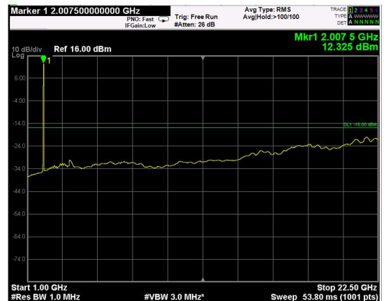
Channel: MIDDLE, Modulation: 256QAM, BW=20MHz, Range: Upper
