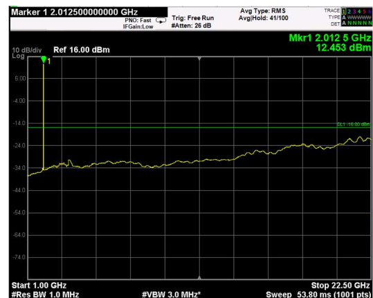
Channel: TOP, Modulation: 16QAM, BW=15MHz, Range: Upper
