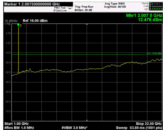
Channel: MIDDLE, Modulation: QPSK, BW=15MHz, Range: Upper
