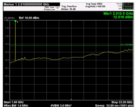
Channel: TOP, Modulation: 64QAM, BW=20MHz, Range: Upper
