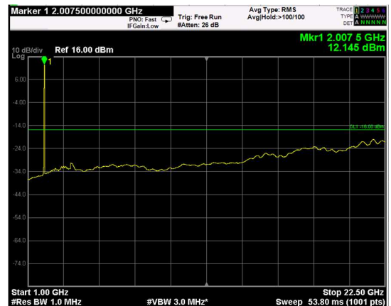
Channel: MIDDLE, Modulation: 64QAM, BW=20MHz, Range: Upper
