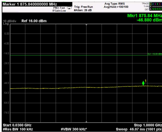
Channel: BOTTOM, Modulation: QPSK, BW=20MHz, Range: Lower
