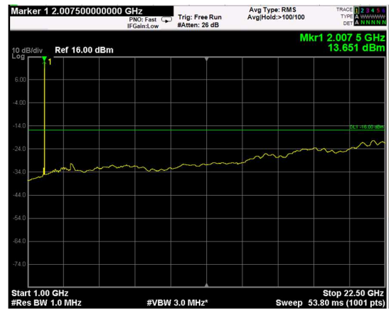
Channel: MIDDLE, Modulation: 64QAM, BW=5MHz, Range: Upper
