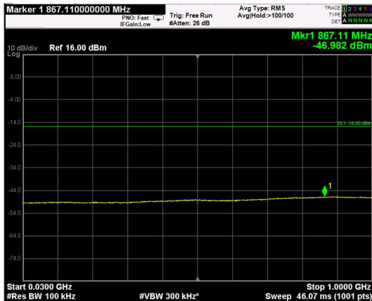
Channel: MIDDLE, Modulation: 64QAM, BW=15MHz, Range: Lower
