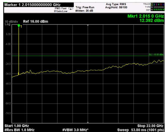
Channel: TOP, Modulation: 16QAM, BW=10MHz, Range: Upper
