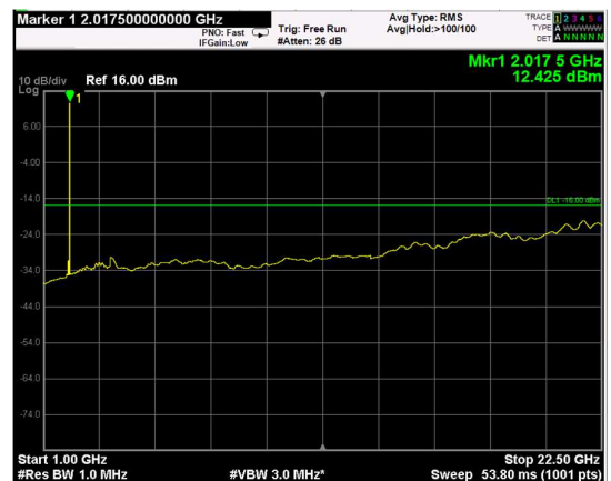
Channel: TOP, Modulation: 64QAM, BW=5MHz, Range: Upper
