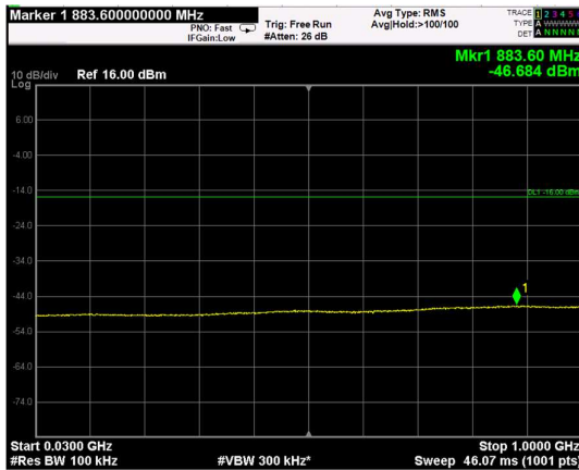
Channel: MIDDLE, Modulation: QPSK, BW=20MHz, Range: Lower
