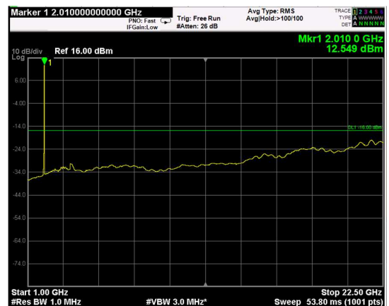
Channel: TOP, Modulation: 256QAM, BW=20MHz, Range: Upper
