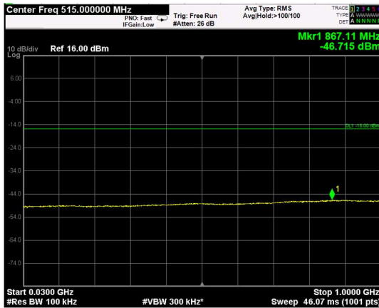
Channel: MIDDLE, Modulation: 16QAM, BW=20MHz, Range: Lower
