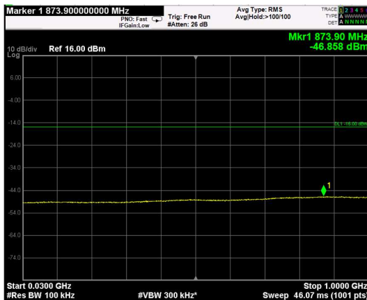
Channel: MIDDLE, Modulation: 256QAM, BW=15MHz, Range: Lower
