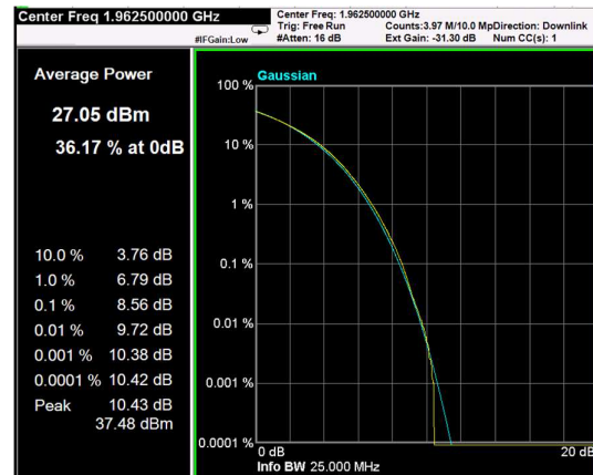
Channel: MIDDLE, Modulation: 16QAM, BW=5MHz, CCDF
