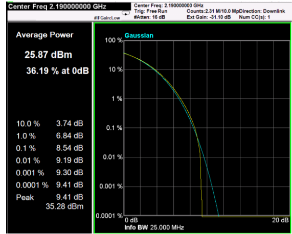
Channel: MIDDLE, Modulation: 256QAM, BW=20MHz, CCDF
