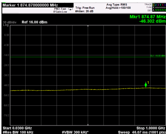
Channel: TOP, Modulation: 64QAM, BW=15MHz, Range: Lower
