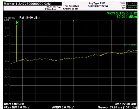
Channel: TOP, Modulation: QPSK, BW=15MHz, Range: Upper
