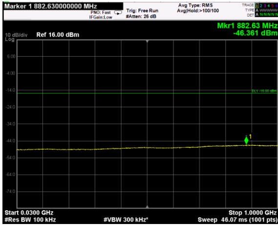
Channel: BOTTOM, Modulation: 64QAM, BW=15MHz, Range: Lower
