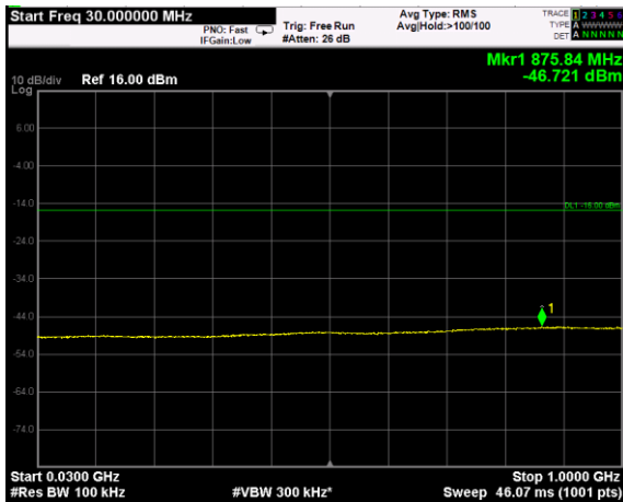
Channel: MIDDLE, Modulation: 256QAM, BW=10MHz, Range: Lower
