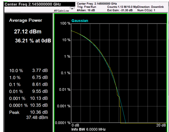
Channel: MIDDLE, Modulation: 16QAM, BW=5MHz, CCDF
