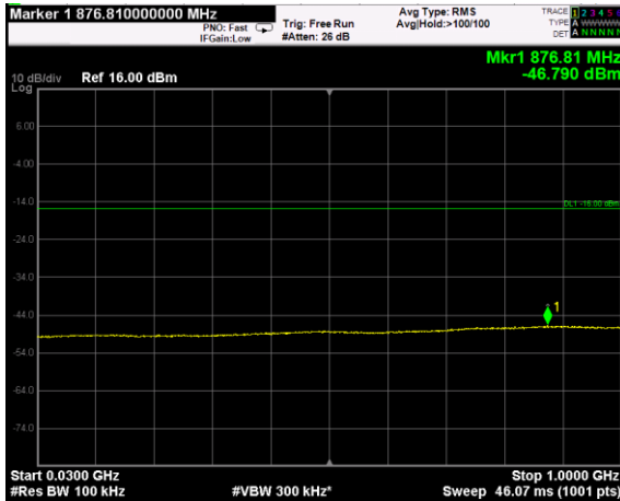
Channel: BOTTOM, Modulation: QPSK, BW=15MHz, Range: Lower
