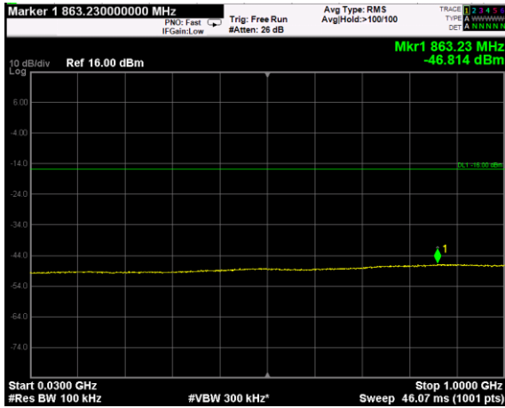
Channel: BOTTOM, Modulation: 256QAM, BW=15MHz, Range: Lower
