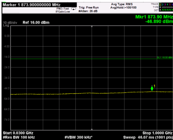
Channel: TOP, Modulation: QPSK, BW=20MHz, Range: Lower
