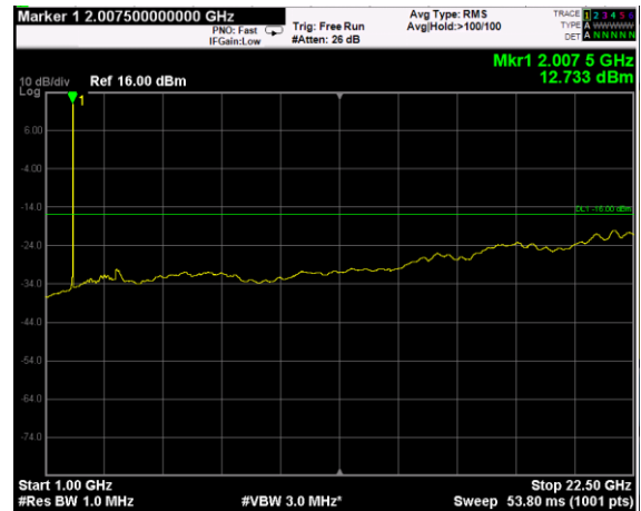
Channel: MIDDLE, Modulation: 16QAM, BW=15MHz, Range: Upper
